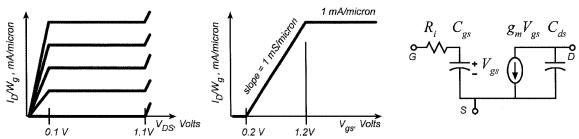
A MOSFET has large-signal parameters as given above and small-signal parameters as given below:
