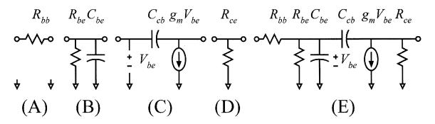
Examining the figure above, we note that network E can be represented as a cascade of networks A-D. Note also that it can be easily shown that  $S_{21}/S_{12} = Y_{21}/Y_{12}$  for any 2-port network.
