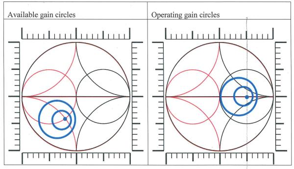
A FET in common-source mode has operating and available gain circles as shown. Find the optimum generator and load impedances (in complex Ohms).
