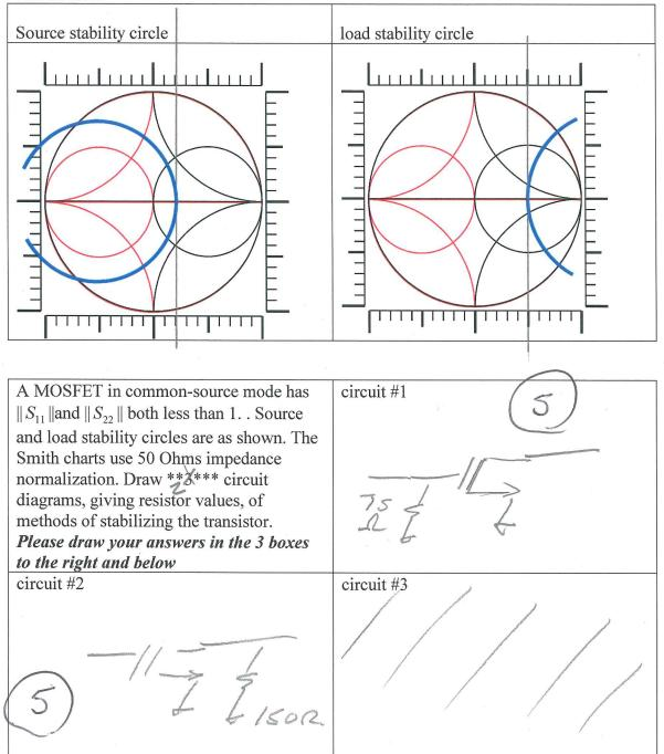
Source > Inside of circle is stalle! Source stesility circle - hits line D= +0,2  $\Rightarrow \frac{1}{2} = \frac{1+0.2}{1-0.2} = \frac{1.2}{0.8} \Rightarrow \frac{1}{2} = \frac{0.8}{1.2}$ => 1/parallel = 0.8 117 SUN SEN 0.8: = 750 ] 75 s gardlet leady 71  $| locd \rightarrow autside | s stable |$  | Circle | hits | hie | Lie = 0.5 |  $| = 3 = 1 + 0.5 = 3 = 7 | y = \frac{1}{3} |$ => /perellel = 3 . son son 3 = 1500 1 => 1500 parellel leading
