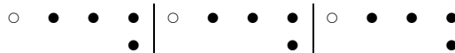
Fig. 13. A canonical WBS encoding of an extended hybrid-redundant number system with the symmetric digit set [-8, 8] .
