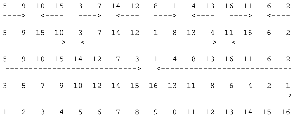
Fig. 14.3. Sorting an arbitrary sequence on a linear array through recursive application of bitonic sorting.
