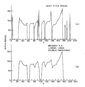
Fig. 14. Effects of the combination smoother on a second pitch period contour with gross errors in the data.
