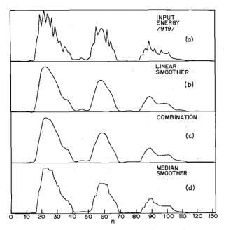
Fig. 8. Effects of linear, combination, and median smoothers on speech input energy for the sequence /919/.
