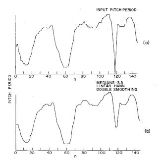
Fig. 12. Effects of the combination smoother on the pitch period contour for a synthesis experiment.
