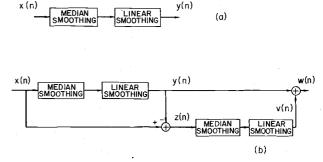
Fig. 4. Block diagrams of smoother and double-smoothing algorithms.
