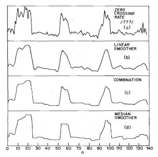
Fig. 9. Effects of linear, combination, and median smoothers on speech zero-crossing rate for the sequence /777/.
