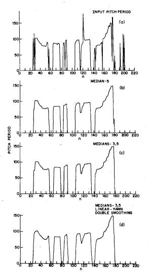
Fig. 13. Comparison of two median smoothers and the combination smoother for a pitch period contour with gross errors.
