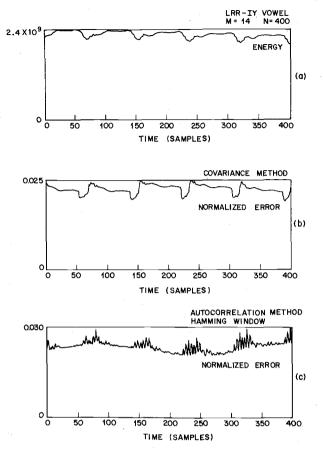
Fig. 7. Prediction-error sequences for N = 400 sample frames.
