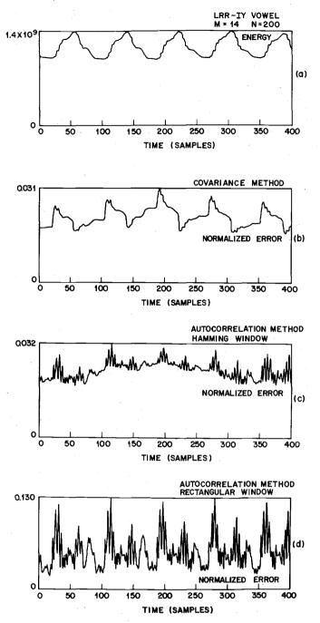
Fig. 6. Prediction-error sequences for 200 samples of speech for three LPC systems.
