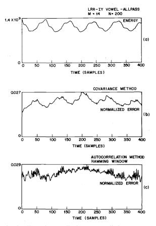
Fig. 10. The effects of allpass filtering on the prediction-error sequence.
