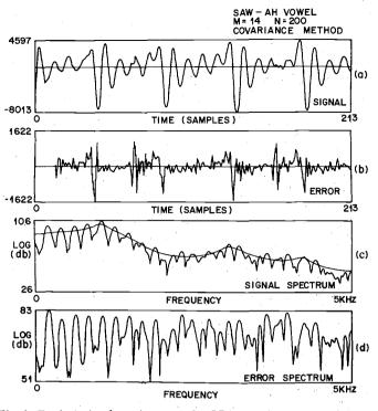
Fig. 4. Typical signals and spectra for LPC covariance method for a female speaker.
