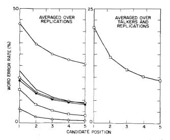
Figure 2 a) Average word error rate for each talker as a function of word position; b) grand average word error rate as a function of word position.
