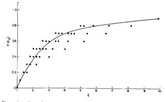
Figure 1 Plot of average word error rate as a function of average word complexity for all possible combinations of a 10-word vocabulary. The smooth curve is a hand drawn curve, which approximates the average behavior of the data.
