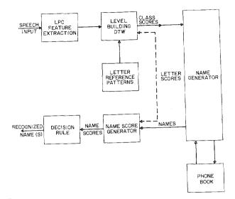
Fig. 3 Block diagram of automatic directory listing retrieval system based on connected letter spelling of names.
