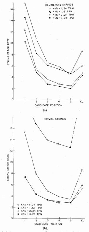
Fig. 3. String error rate versus candidate position for the four recognition tests for (a) deliberate strings, and (b) normal rate strings. The individual symbols denote measured error rates for the different KNN rules, and for the specified number of templates per word (TPW).
