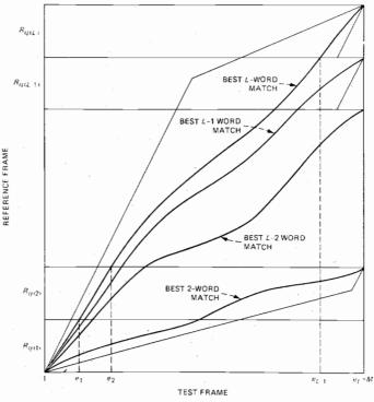
Fig. 2. Sequence of level building DTW warps to provide best word sequences of several different lengths.
