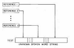
Fig. 1. Illustration of connected word recognition by concatenation of individual reference patterns.
