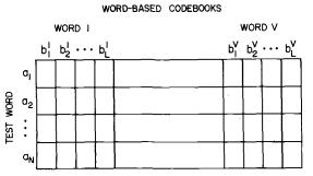
Fig. 3. Distance computation in the word-based VQ preprocessor. By saving each individual distance computation in a table, a reduction in quantization error in the DTW stage is achieved.
