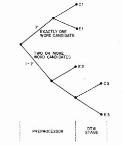
Fig. 5 A breakdown of the potential sources of error in the preprocessor and in the DTW stage of the recognizer.
