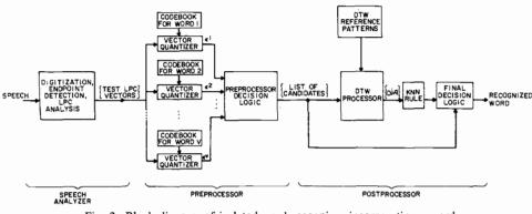
Fig. 2. Block diagram of isolated word recognizer incorporating a wordbased VQ preprocessor and a DTW-based postprocessor.
