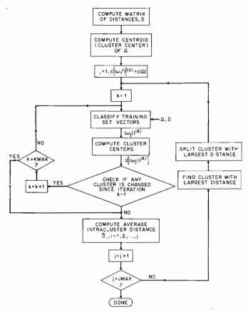
Fig. 2. Flow diagram of the MKM clustering procedure.
