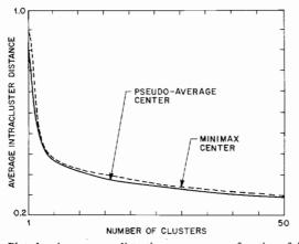
Fig. 3. Plot showing average distortion measure as a function of the number of clusters used per word for the minimax center (dotted-line) and the pseudoaverage center (solid line).
