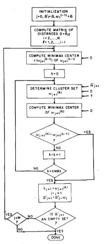
Fig. 1. Flow diagram of the UWA clustering procedure.
