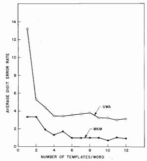
Fig. 4. Average digit error rate versus the number of templates per word for a laboratory database of 1000 digits with clusters generated by both the UWA and MKM clustering procedures.
