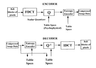
Fig. 2. Block diagram of JPEG encoder and decoder.
