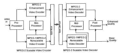
Fig. 8. Generalized codec for MPEG-2 scalable video coding.
