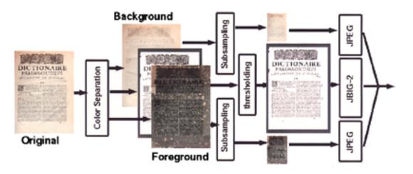
Fig. 4. DJVU compression algorithm first runs the foreground/background separation. Both the foreground and background images are compressed using a sparse wavelet encoding dubbed IW44, while the binarized text and drawings are compressed using AT&T's proposal to the JBIG2 standards committee.
