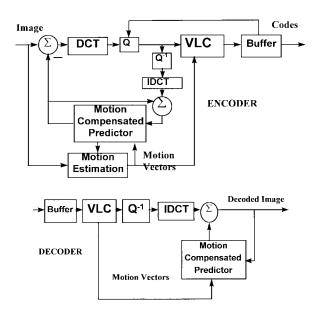
Fig. 6. Motion compensated codec for interframe coding.
