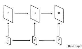
Fig. 14. Spatial scalability with two layers (courtesy MPEG Video Group).
