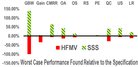
Figure 9: Worst-case performances relative to the specifications found by HFMV and SSS in the \pm 8\sigma region.
