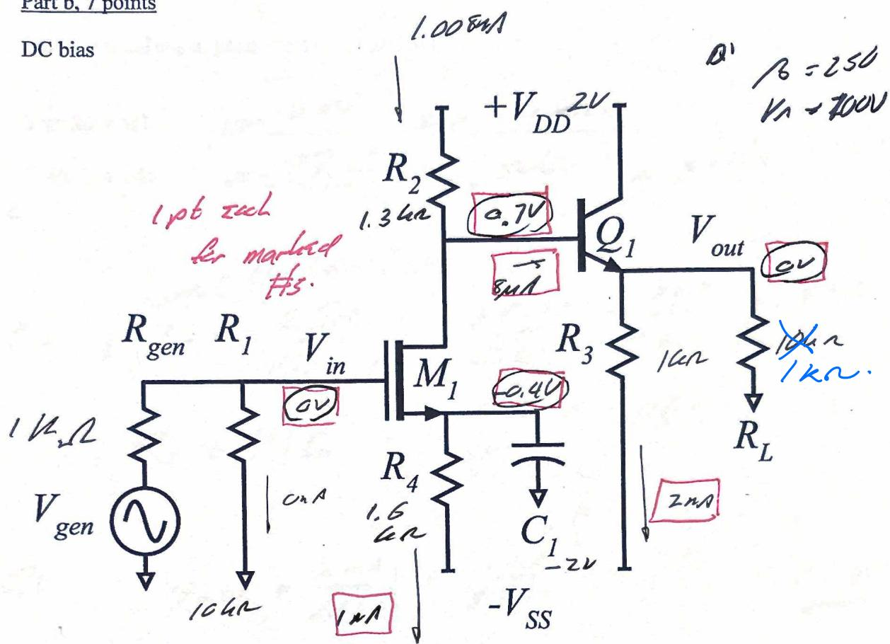
On the circuit diagram above, label the DC voltages at ALL nodes and the DC currents through ALL resistors
