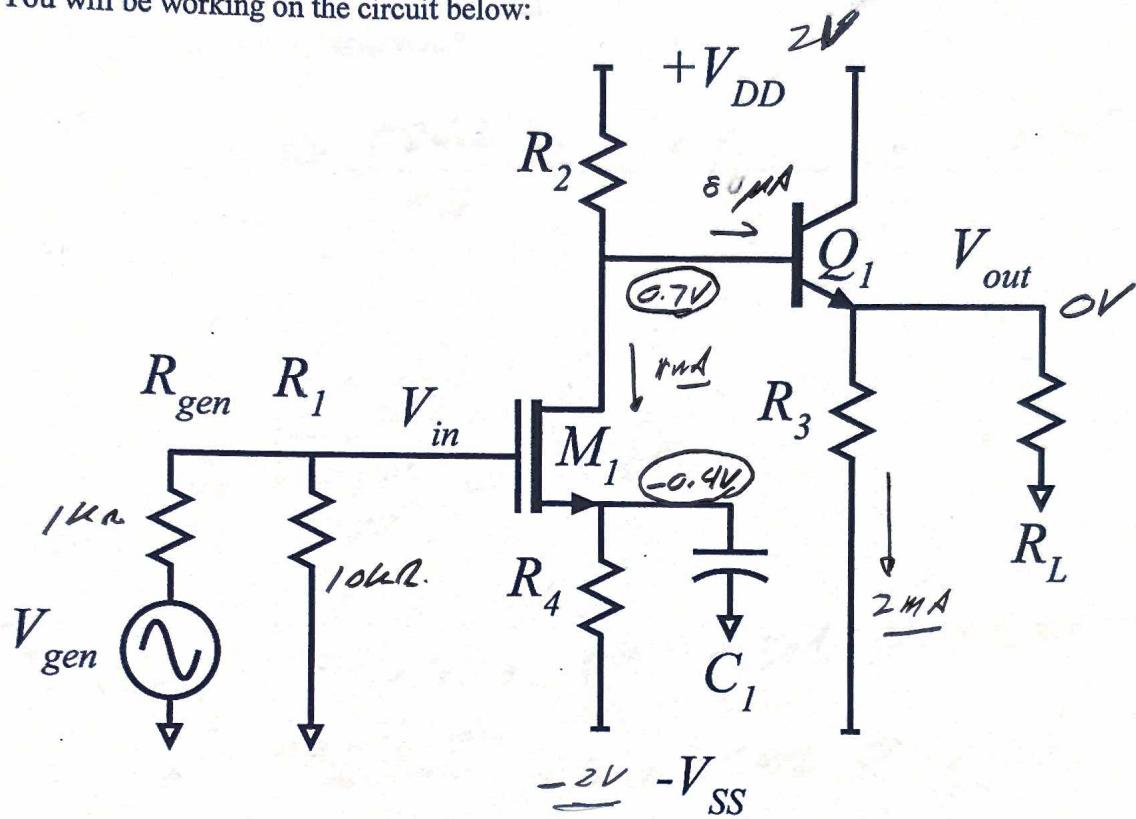
$$M1: K_\mu = \mu c_{gs} W_g / 2L_g = 10 \text{ mA/V}^2 \cdot (W_g / 1 \mu\text{m})$$
