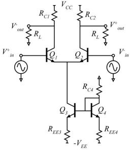
Problem 4 The circuit now uses a constant current source to bias the differential amplifier. For Q1 and Q2 the DC collector voltages and DC collector currents remain the same as in problem 2. There is a 0.30 V IR drop across Ree3, while the DC current in REE4 is 1/10th of the emitter current of REE3. Find all resistor values. Find the bias conditions, the differential and common-mode gains, and the commonmode rejection ratio. The diode has the same "on" voltage as the transistors.
