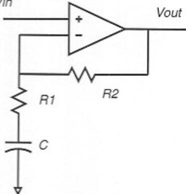
The amplifier has a differential gain of  $10^6$ .
