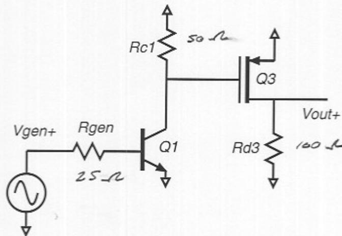
Because the input is fully differential, with  $V_{gen+} = -1 * V_{gen-}$ , the circuit can be analyzed using a half-circuit equivalent.
