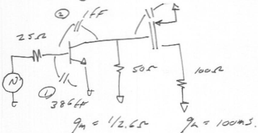
$$R_{11}^0 = 25\Omega \quad R_{11}^0 C_1 = 25\Omega \cdot 386\text{fF} = 9.65\text{ps}$$
