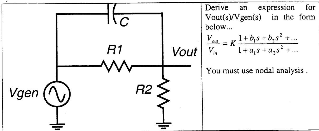
$$V_{out}(s)/V_{gen}(s) = \frac{\left( \frac{R_2}{R_1 + R_2} \right) \left( \frac{1 + sR_1 C}{1 + s[R_1 || R_2]C} \right)}{1}$$
