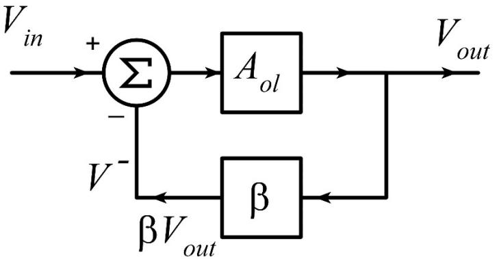
We have seen that if  $T(s)$  has 3 or more poles, the system can be unstable if the magnitude of the loop transmission is sufficiently large.
