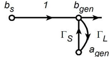
Power delivered to a matched load  $\Gamma_L = \Gamma_S^*$
