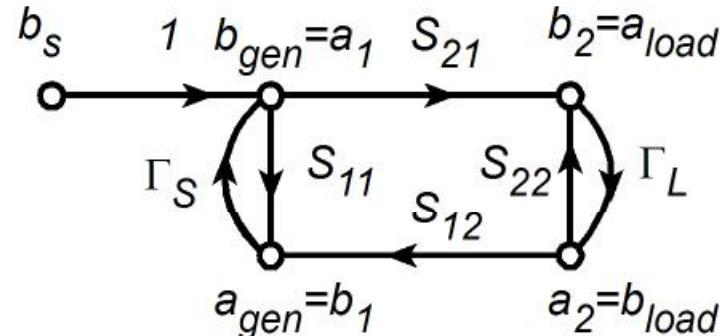
$$\frac{a_{load}}{b_s} = \frac{S_{21}}{1 - \Gamma_s S_{11} - \Gamma_l S_{22} - \Gamma_s \Gamma_l S_{21} S_{12} + \Gamma_s S_{11} \Gamma_l S_{22}} = \frac{S_{21}}{(1 - \Gamma_s S_{11})(1 - \Gamma_l S_{22}) - \Gamma_s \Gamma_l S_{21} S_{12}}$$
