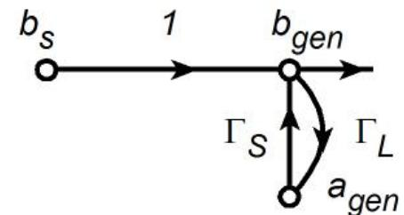
so :  $\|b_{gen}\|^2 = \frac{\|b_s\|^2}{\|1 - \Gamma_s \Gamma_L\|^2} \quad \text{and} \quad \|a_{gen}\|^2 = \|\Gamma_L\|^2 \cdot \|b_{gen}\|^2$
