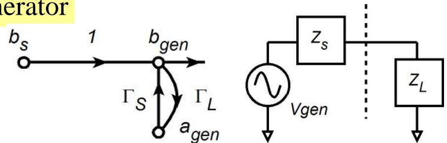
We must now match on input and output :  $\Gamma_S = S_{11}^*$  and  $\Gamma_L = S_{ss}^*$
