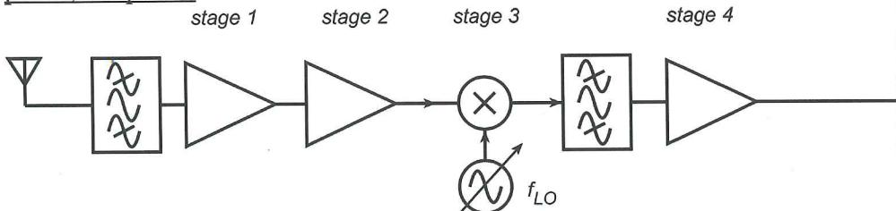
Given the radio block diagram above, the IF frequency is 10 MHz and the (tunable) LO frequency is placed \*below\* the input RF frequency. This is a very low-data-rate receiver, hence the IF filter is very narrow, only  $\pm$  10 kHz bandwidth. The RF preselect filter is not tunable. If the receiver's RF tuning range has a lower limit of 500 MHz, what is the highest frequency to which the receiver can be tuned if image responses are to be avoided?
