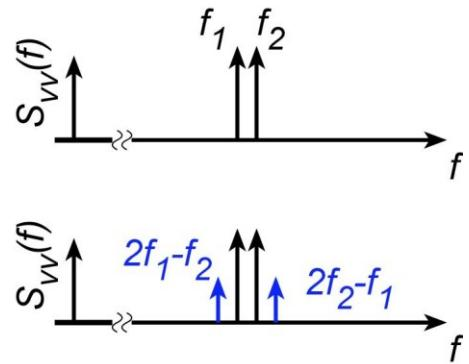
We will soon show that, given \*odd - order distortion\*, strong input signals at frequencies  $f_1$  and  $f_2$  will generate distortion tones at frequencies  $(2f_1 - f_2)$  and  $(2f_2 - f_1)$ .
