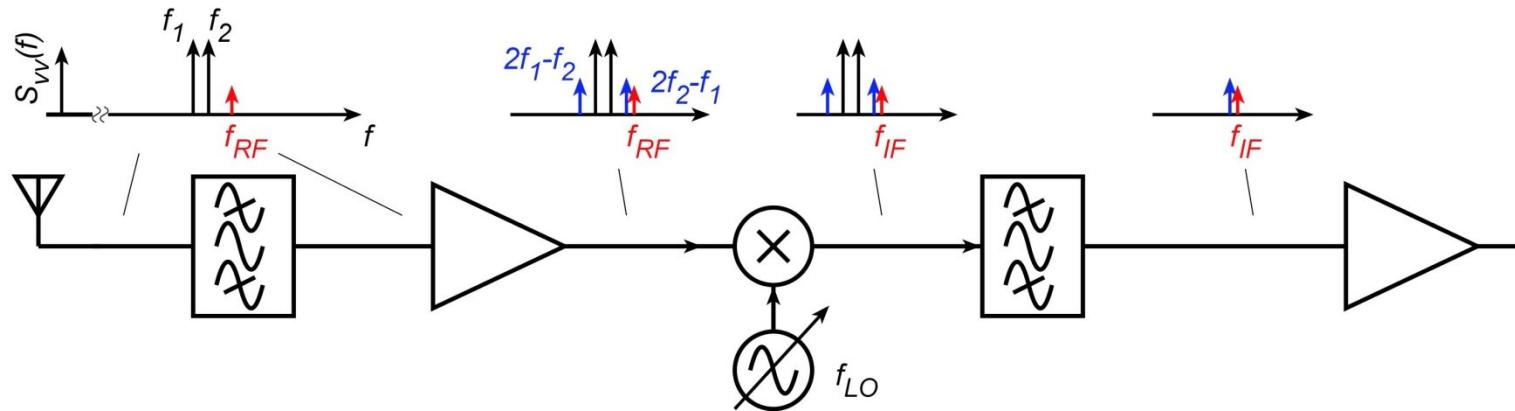
If the tones at  $f_1$  and  $f_2$  lie outside the passband of the RF filter, they will be rejected, and the receiver will suffer no interference.
