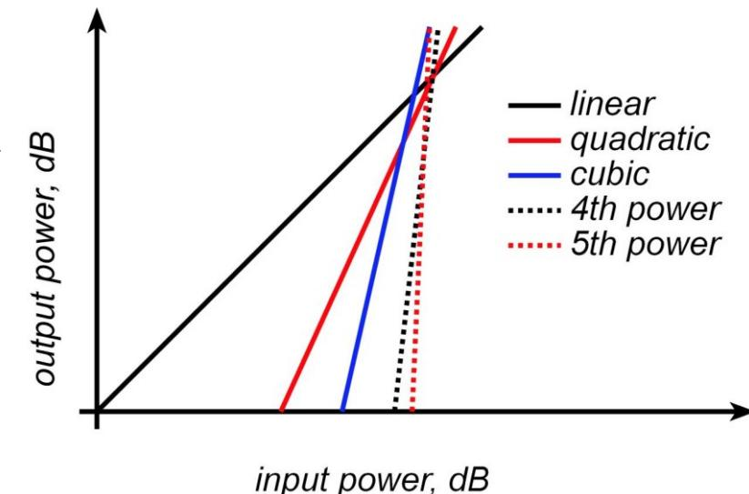
But the power at  $(2\omega_1 - \omega_2), (2\omega_2 - \omega_1)$  involves 3<sup>rd</sup>, 5<sup>th</sup>, 7<sup>th</sup> order terms, and varies with 3 : 1 slope only at low inputs where the cubic term dominates.
