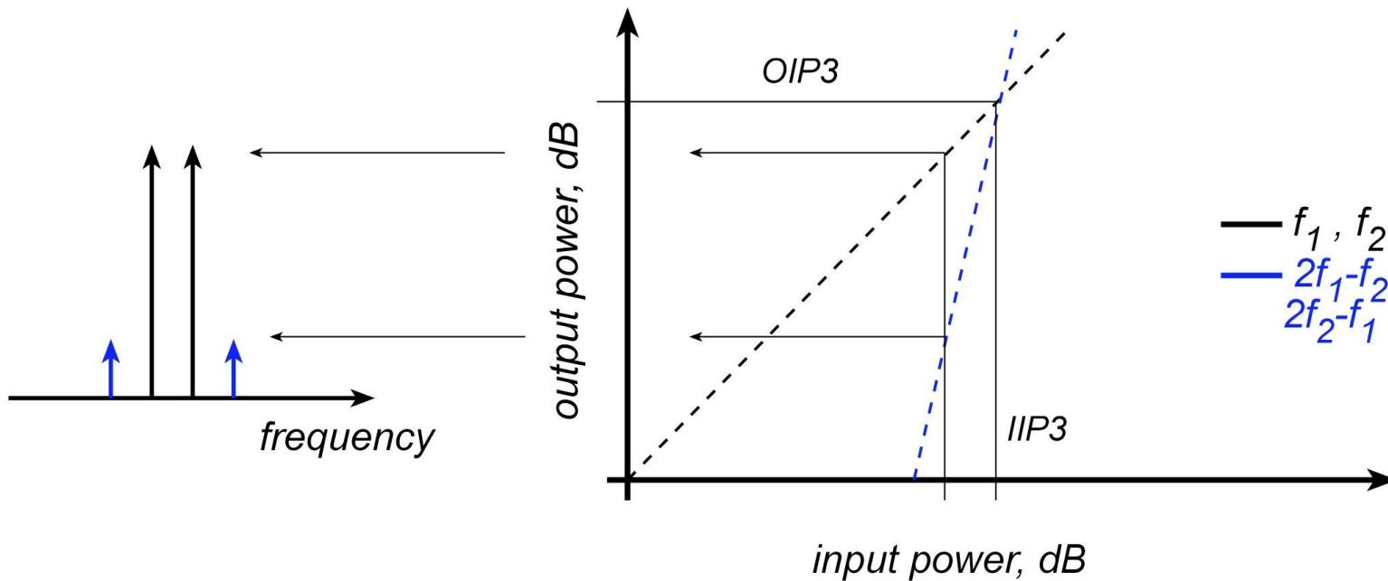
3rd - Order distortion has 3 : 1 slope on log - log (dB) plot:
