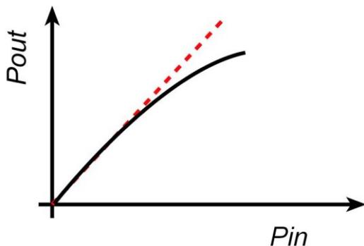
The above assumes a cubic-only model, i.e. that the  $V_{in}^5$ ,  $V_{in}^7$ , etc. terms are negligible. In general, this is \*not\* a good assumption for an amplifier approaching hard clipping
