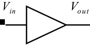
$2^{\text{nd}}$  - order response: outputs at  $\pm n\omega_1 \pm m\omega_2$ , with  $n + m = 2$
