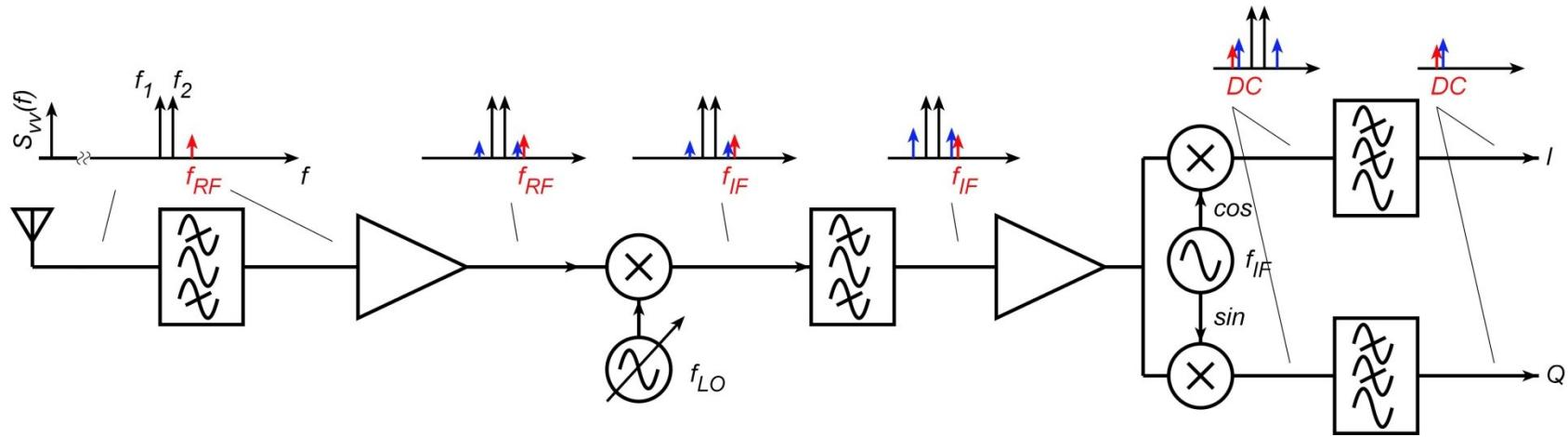
In a dual - conversion receiver, the strong interferers at  $f_1$  and  $f_2$  may lie inside the passbands of both the RF \* and \* IF filters.
