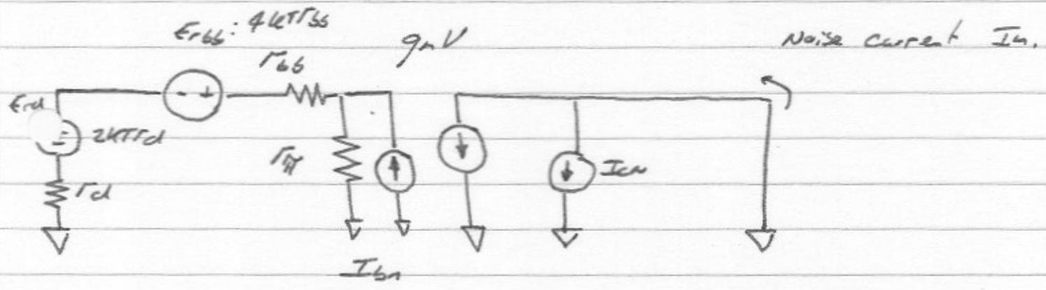
$$I_n = (E_{rd} + E_{rs}) \cdot \frac{r_{\pi}}{r_{\pi} + r_d + r_{bb}} \cdot g_m$$
