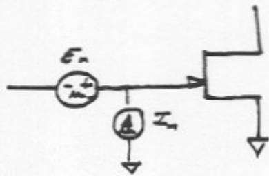
~~$\frac{d\langle E_n^2 \rangle}{df} = 4KT r_1 + \frac{4KT \Gamma}{g_m} (1 + (2\pi f C_{gs})^2 r_1^2)$~~
