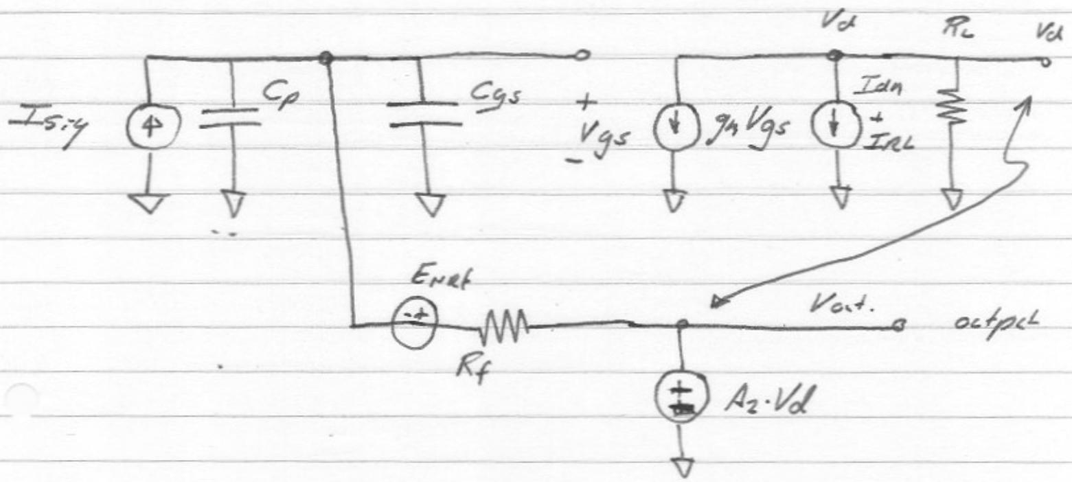
This is the model of a pin-fet optical receiver preamplifier.
