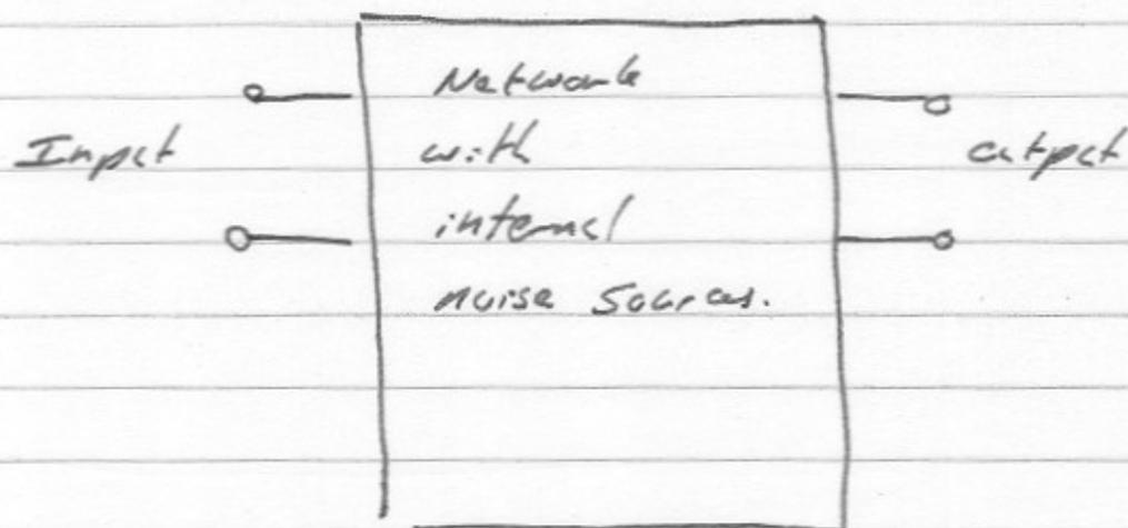
We desire to analyze the network to find the input-referred noise (voltage/current/power etc)
