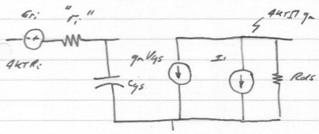
this model lumps  $r_i + r_s + r_y \rightarrow r_i$
