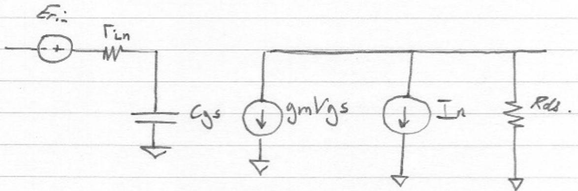
$$\left. \begin{aligned} E_{r,i}: S &= 4kT\Gamma_{L,i} \\ I_n: S &= 4kT\Gamma_{I_n}g_m \end{aligned} \right\} \text{zero cross-spectral density.}$$
