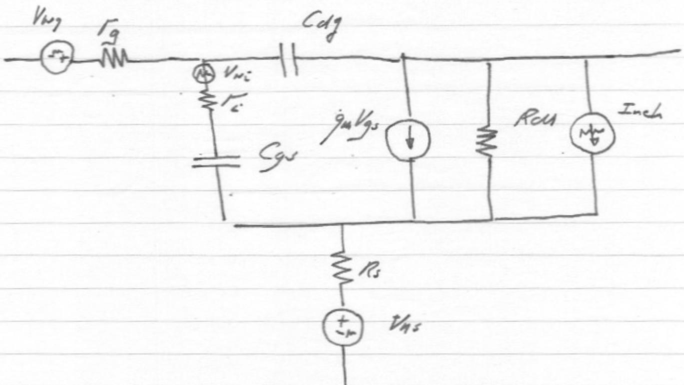
where  $V_{ng}$ ,  $V_{ns}$ , are thermal noise generators for
