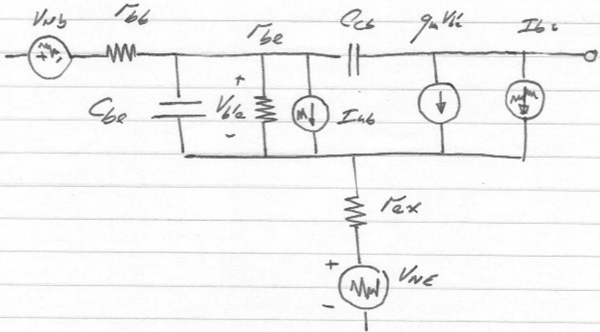
where  $V_{Nb}$  &  $V_{ne}$  are the thermal noise
