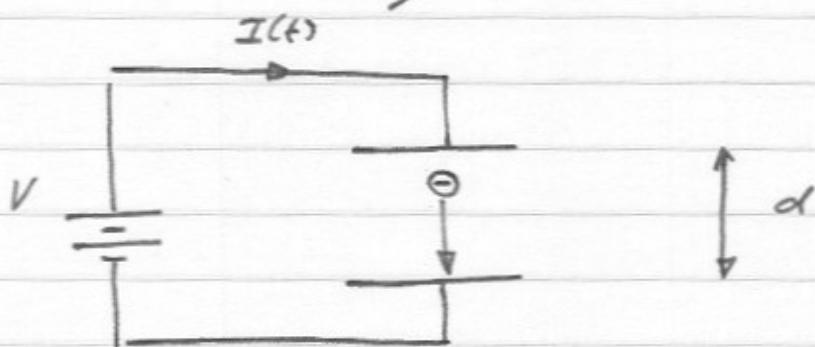
with an electron moving between the plates of a capacitor of separation  $d$ , Energy balance consideration between the electron electrostatic potential ( $\int E \cdot dk$ ) and the circuit energy ( $\int V \cdot I(t) dt$ ) results in
