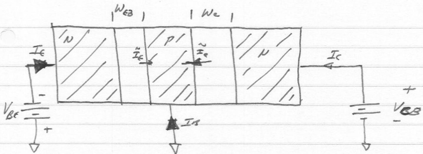
we are forcing  $V_{BE}$  &  $V_{CE}$  to be fixed dc. voltages. Therefore in our base-diffusion equivalent circuit model, we are forcing the electron concentrations at the 2 boundaries:
