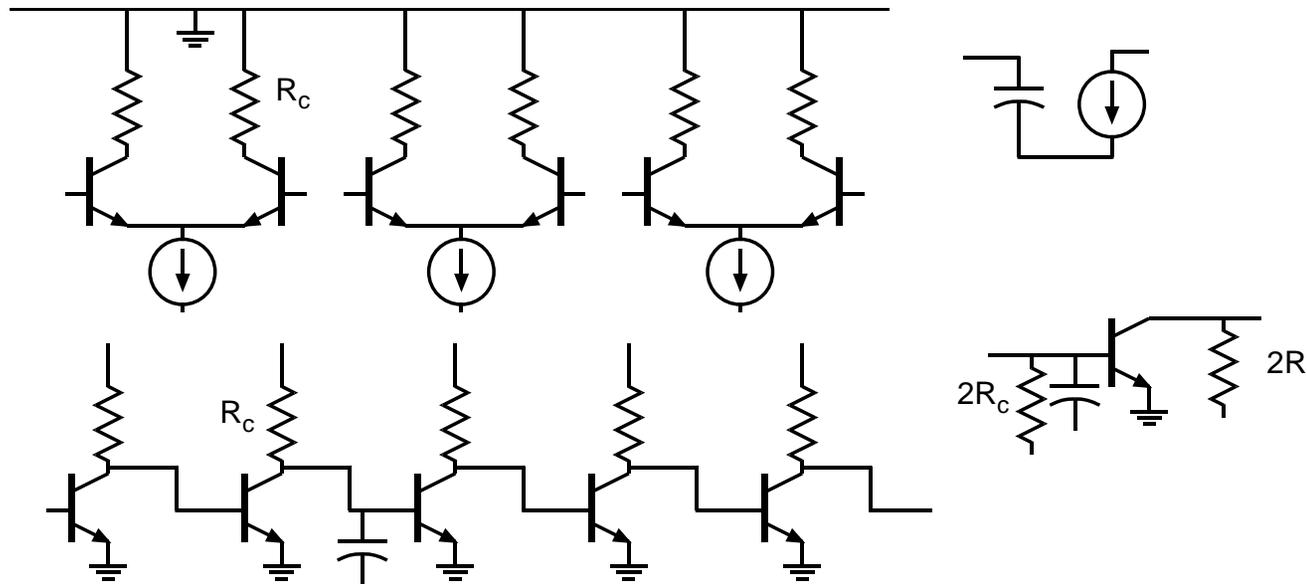
Examine a cascade of simple differential pairs. For the differential signal path, this becomes a CE stage cascade. If we model each BJT as a simple  $g_m$  &  $C_{in}$  combination, the gain per stage is  $-g_m R_C$ , the bandwidth is  $1/2\pi R_C C_{in}$ , and the gain - bandwidth product is  $g_m / 2\pi C_{in} = f_\tau$ . This is the origin of the " $f_\tau$  limit". We can do much better.
