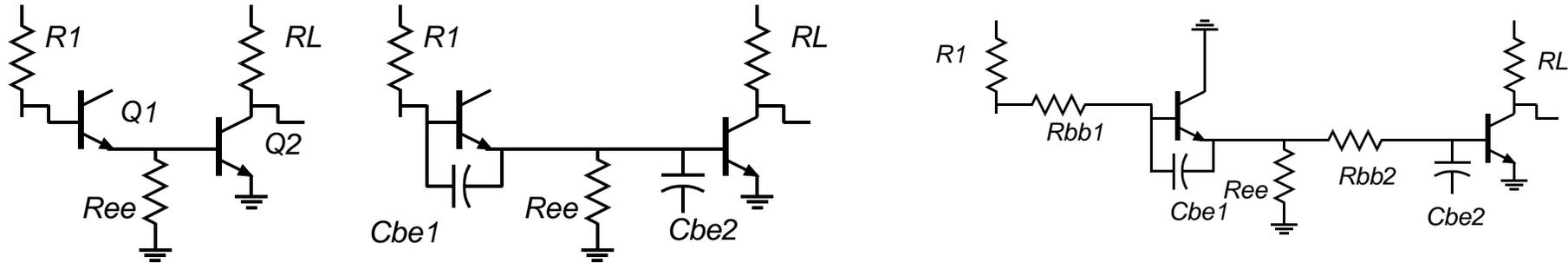
Addition of  $R_{ee}$  has 2 effects. The  $Q_1$  EF gain is reduced
