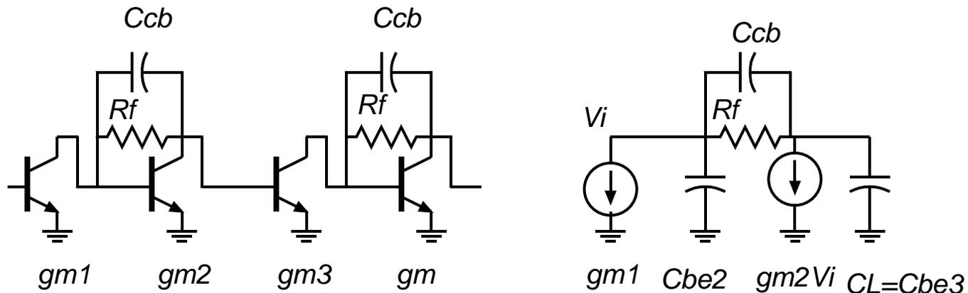
$$a_1 = C_{be2} / g_{m2} + C_{be3} / g_{m2} + C_{cb} R_f$$
