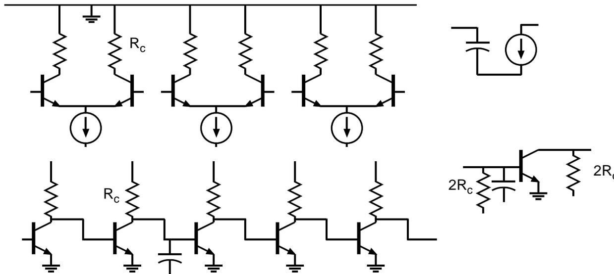
Let us think this through. Transistors are made to provide transconductance  $g_m$ . An input voltage is converted into an output current. Our simplest design strategy is to convert this output current back into a voltage using a resistor...hence the gain relationship. Transconductance \* always \* comes at the price of input capacitance, by the ratio  $C_{in} = g_m / 2\pi f_\tau$
