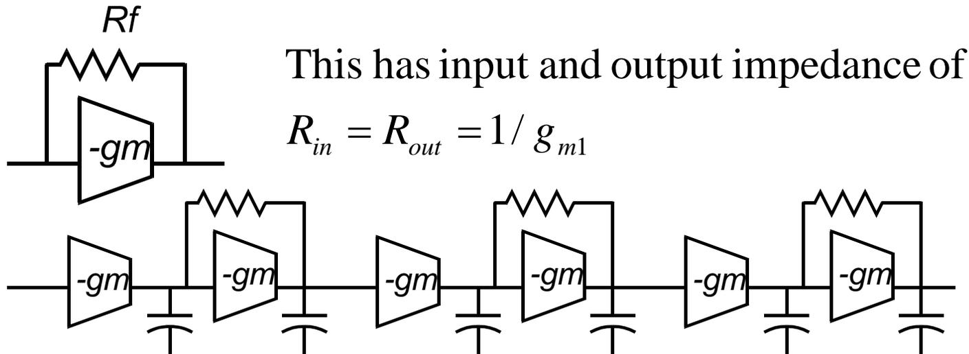
So each capacitor has charging time constant of  $C / g_{m1}$
