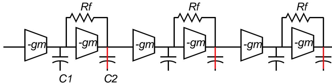
Shorting  $C_2$  makes the  $C_1$  charging time constant  $= C_1 R_f$
