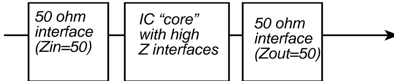
If IC has small dimensions, we can use high -  $z$  internal interfaces, and just interface to e.g. 50 Ohms at chip boundaries or (in some cases) between major circuit blocks on wafer
