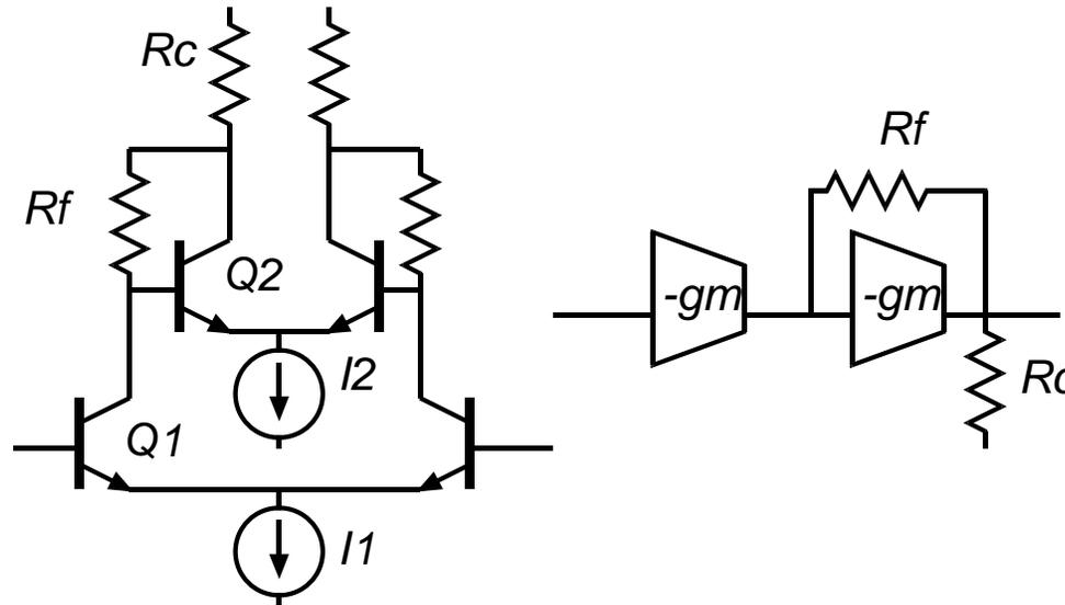
If  $I_1 < I_2$  (derive this) amplifier will always limit on the gm stage, not the Zt stage....hence large - signal operation maintains low impedances (hence short time constants) provided by feedback.
