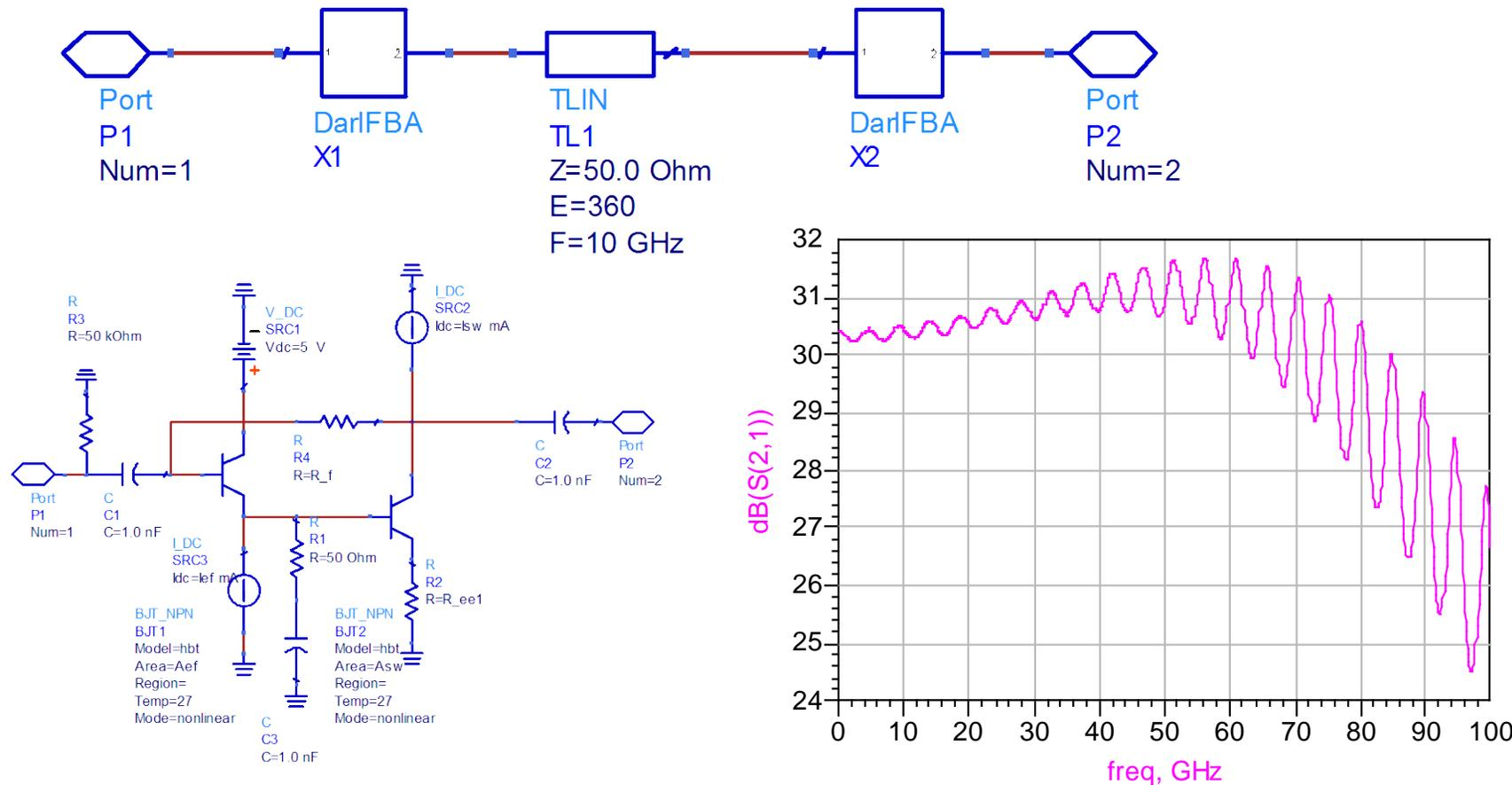
Standing waves on transmission lines cause gain/phase ripples of the form  $(1 - \Gamma_S \Gamma_L \exp(-j2f\tau))^{-1}$ . Either we must have short transmission lines, or the lines must be well-terminated
