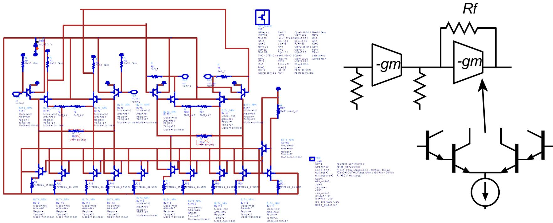
First stage is resistively terminated, second stage has resistive feedback...this is because first stage is allowed to limit, or can have AGC applied, either of which would violate the feedback gain/impedance relationships...
