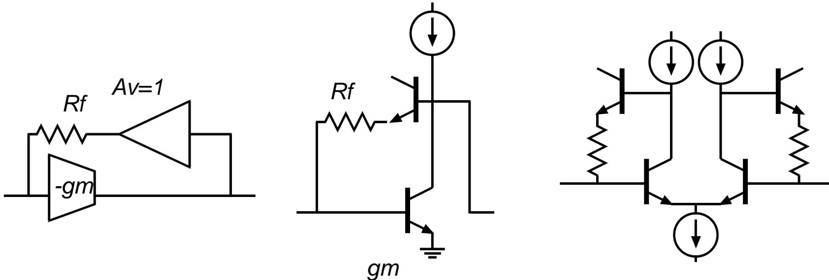
This is often used for ease in biasing . The required  $g_m$  is also reduced to  $g_m = -A / R_{in/out}$  .
