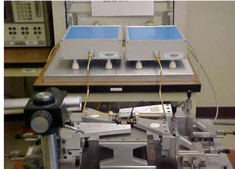
GGB Wafer Probes 330 GHz available with bias Tees
