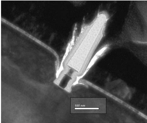
Figure 3: Cross-section of regrown S/D InGaAs FET with a 27 nm gate.
