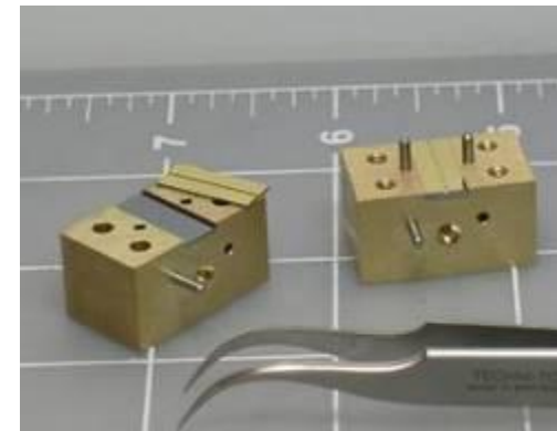
300 GHz oscillator in W/G block under test
