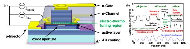
Fig. 1. (a) Schematic of a FICSL showing an intra-cavity electro-thermo tuning region (b) Band diagram showing different current flows
