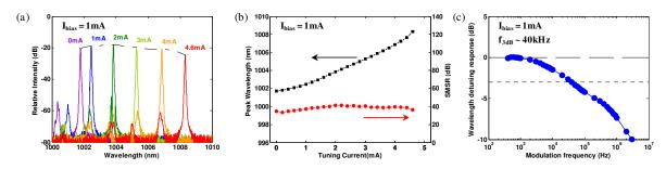
**Fig. 2.** Room temperature wavelength tuning of a 3  $\mu$ m device with  $I_{bias} = 1$  mA (a) lasing spectra with different  $I_{tuning}$ . (b) Peak wavelength and side mode suppression ratio (SMSR) vs.  $I_{tuning}$ . (c) Dynamic tuning characteristics with a cut-off frequency  $f_{3dB} \sim 40$  kHz.
