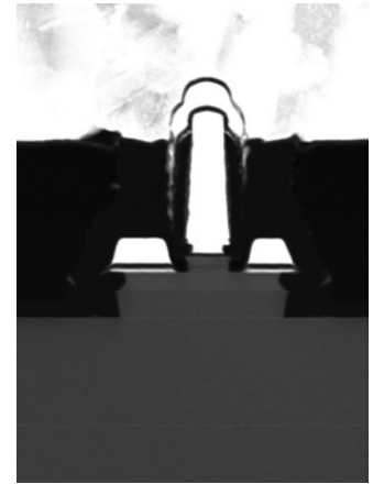
Fig. 2 TEM Cross-section of 130 nm InP HBT. Collector Ohmic contacts are not shown in image.
