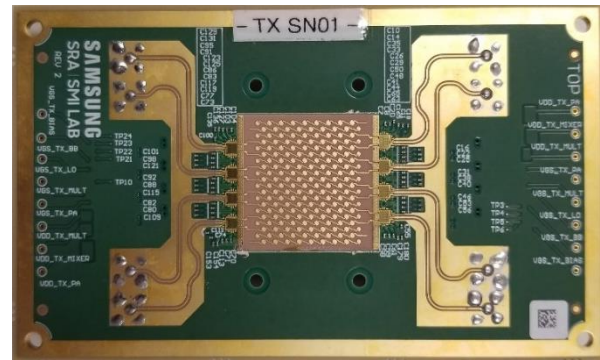
Fig. 3. The TX beamformer module with eight dual-channel 144GHz RFICs wire bonded to the antenna array.
