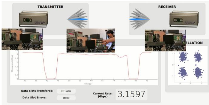
Fig. 15. Demonstrating 3 Gbps link with beam steering.
