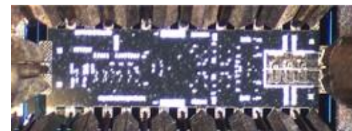
210 GHz RX: measured 27dB gain, 25GHz BW, 8-8.5dB NF.
