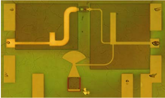
Fig. 3: One-HBT (transferred-substrate) 6.3 dB gain amplifier at 175 GHz
