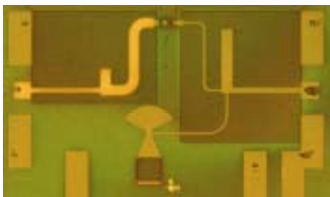
Figure 4: Single-HBT amplifier with 6.3 dB gain at 174 GHz
