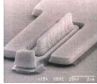
Figure 1: SEM photograph of a typical InP Mesa HBT
