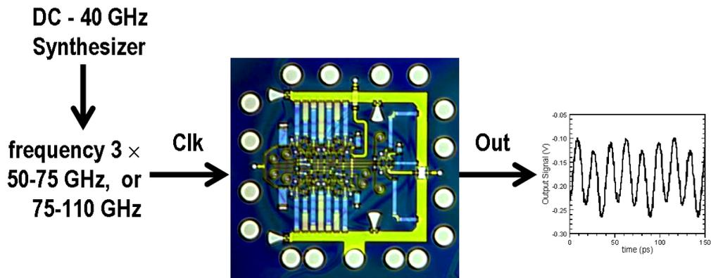
Figure 5.3: 50-75 and 75-110 GHz divider testing
