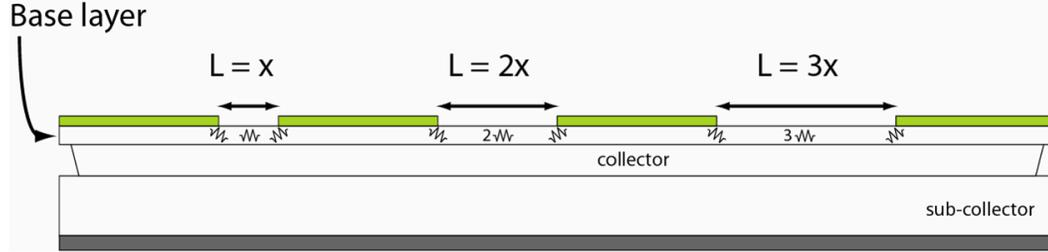
Figure 2.4: Non-pinned TLM structure – the base semiconductor is exposed
