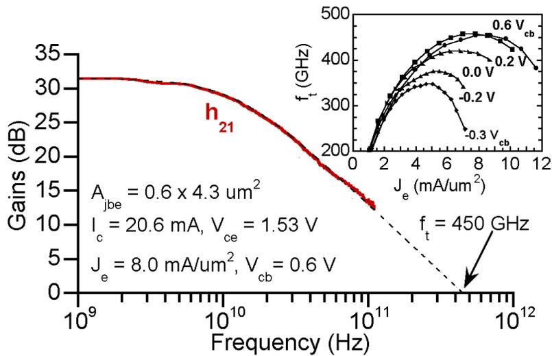
Figure 4.29: Measured microwave gains, DHBT 27 – Peak  $f_\tau$
