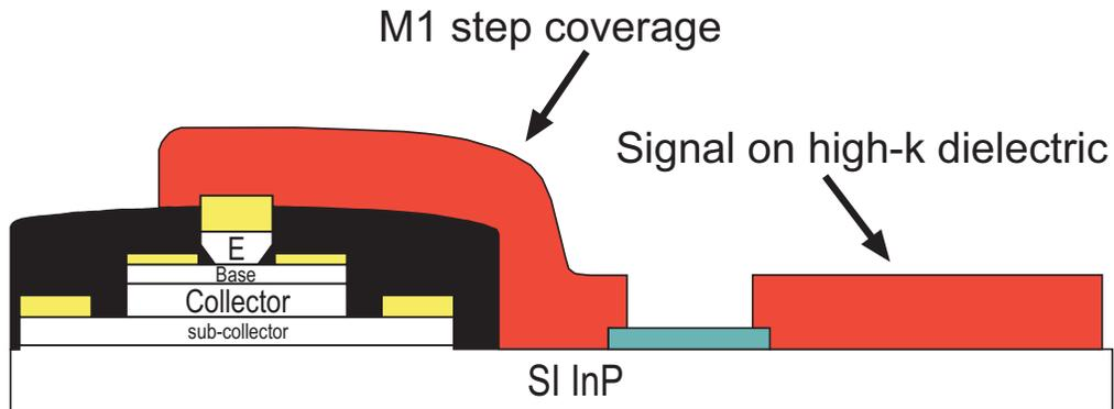
Figure 3.5: Old HBT process after passivation and Metal-1 interconnect
