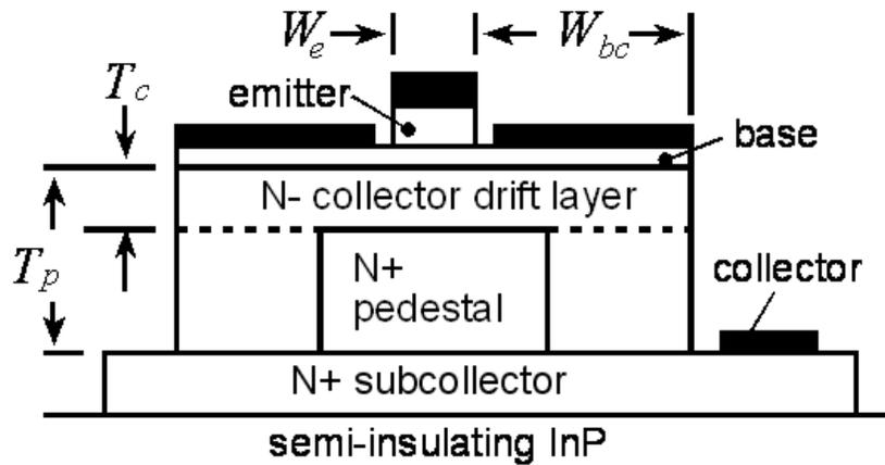
Figure 2.15: Pedestal process schematic
