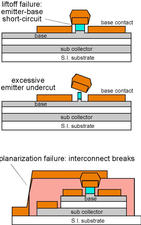
Figure 3.1: Failure mechanisms that limit yield for mesa HBTs
