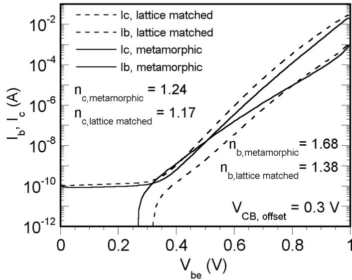
Figure 4.36: Gummel curves – comparing metamorphic and lattice-matched DHBT characteristics
