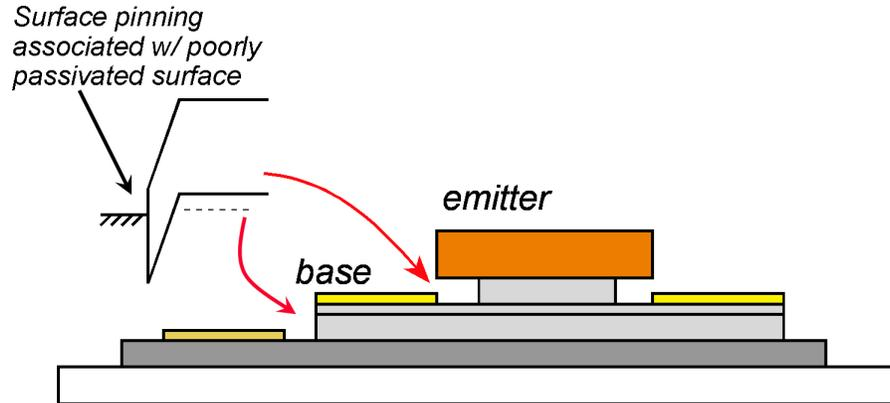
Figure 3.4: Device cross-section showing leakage paths for poorly passivated surfaces
