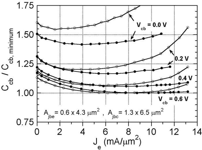
Figure 4.24: Comparison of  $C_{cb}$  vs  $J_e$  and  $V_{cb}$  for both 100 nm collector devices—42 nm transition (DHBT 25) filled, 25 nm transition (DHBT 26) hollow
