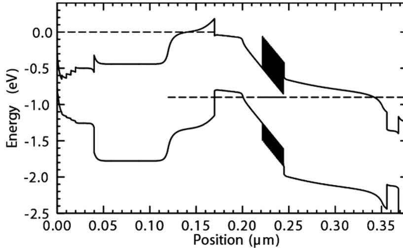
Figure 4.4: Simulated band-structure DHBT 22 –  $V_{be} = 0.9$  V,  $V_{cb} = 0.0$  V
