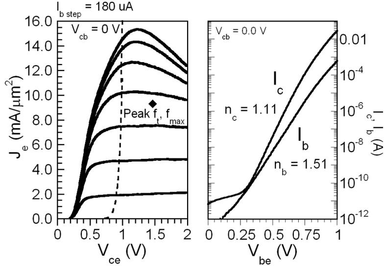
Figure 4.15: Common-emitter I-V and Gummel characteristics, DHBT 26
