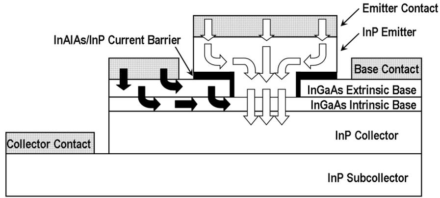
Figure 2.16: Regrown-emitter process schematic
