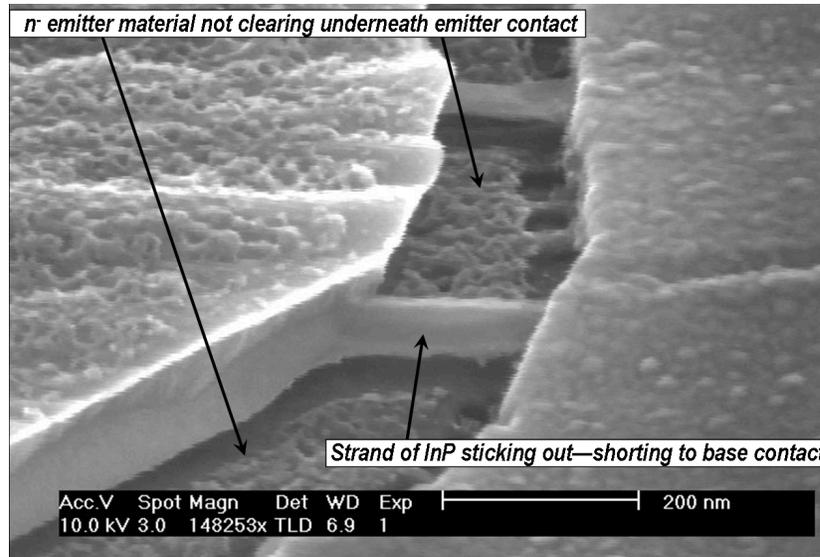
Figure 3.19: Inspection of the  $N^-$  semiconductor between the etched emitter mesa and self-aligned base contact
