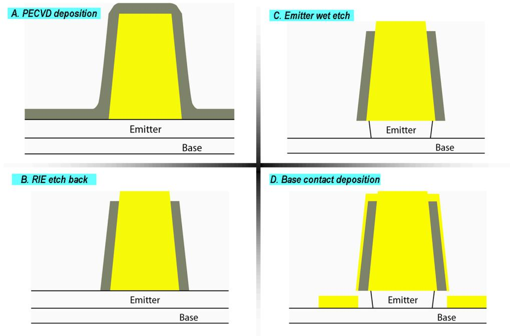
Figure 3.20: Process flow for emitter dielectric sidewall spacer
