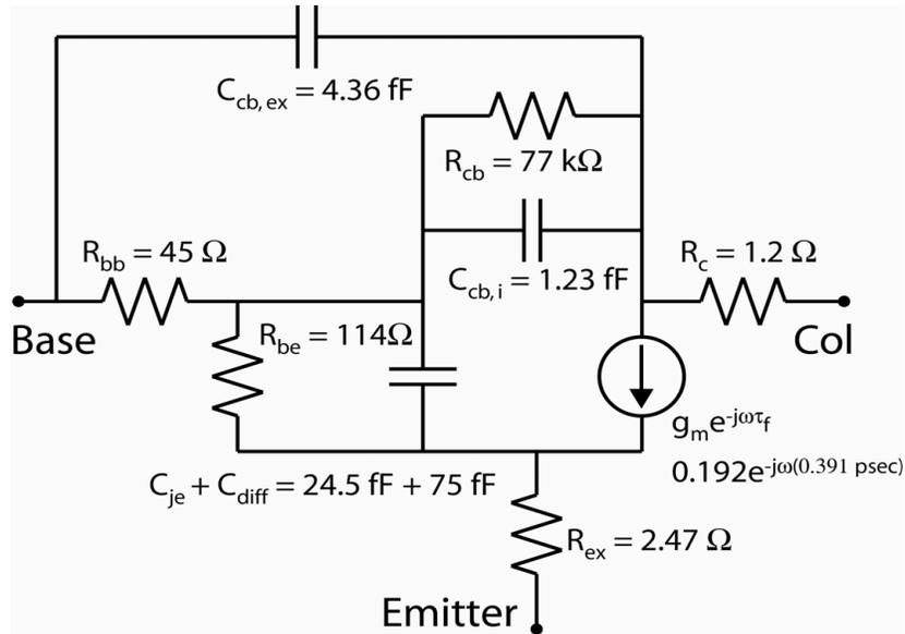
Figure 4.11: Hybrid- $\pi$  model, DHBT 24 – Peak  $f_\tau$ ,  $f_{max}$
