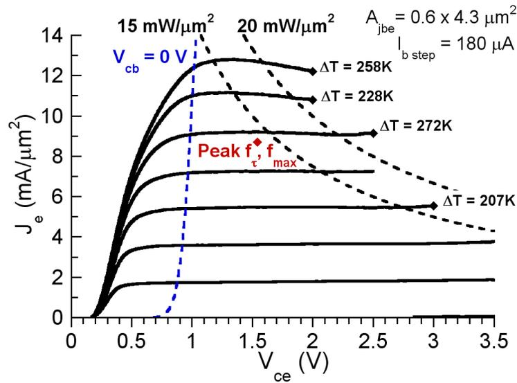
Figure 4.26: Common-emitter current-voltage characteristics, DHBT 27
