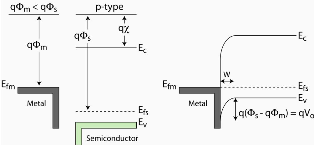
Figure A.1: Band line-up of p-type ohmic contact
