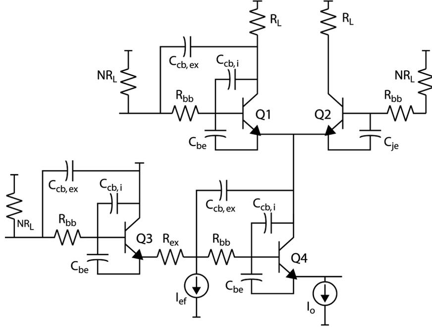
Figure 2.12: Delay path and capacitors charged during clock transition
