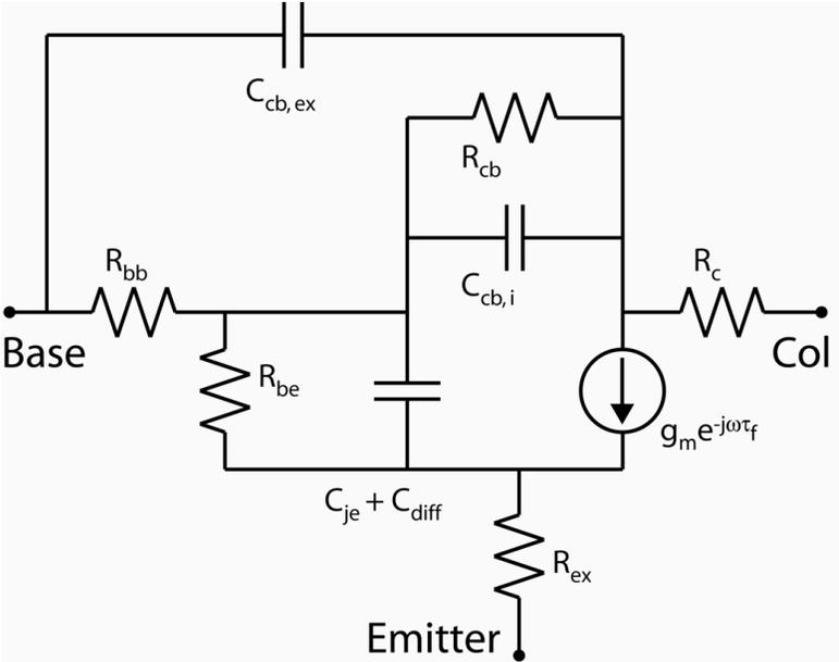
Figure 2.7: Hybrid-pi equivalent circuit HBT model
