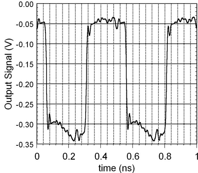
Figure 5.14: UCSB divide-by-2 output waveform,  $f_{clk} = 4$  GHz,  $f_{out} = 2$  GHz
