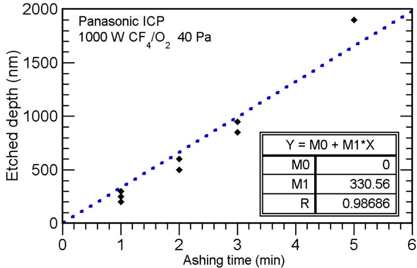
Figure B.1: BCB etch rate for the given CF<sub>4</sub>/O<sub>2</sub> recipe
