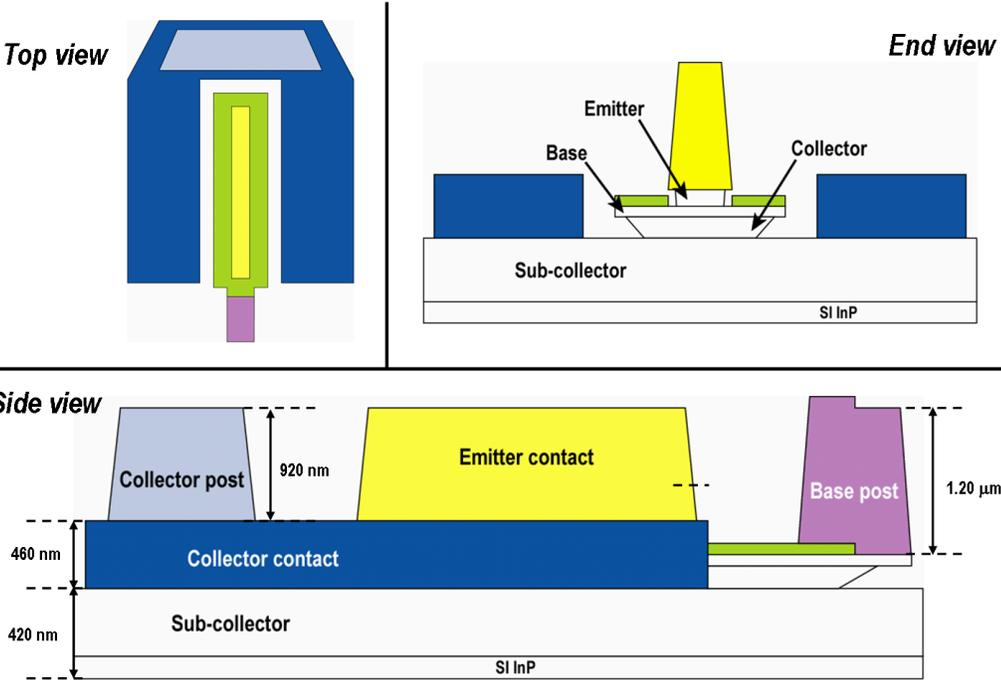
Figure 2.1: Mesa HBT structure w/ self-aligned base contact
