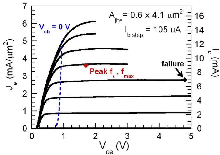
Figure 4.9: Common-emitter I-V characteristics, DHBT 24
