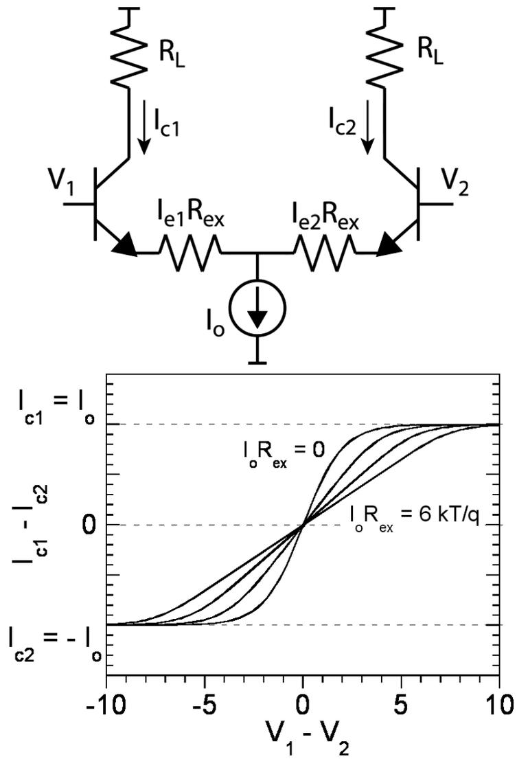
Figure 2.13: Current flow of a differential pair in the presence of emitter resistance –  $I_o R_{ex} = 0, 2kT/q, 4kT/q,$  and  $6kT/q$ .  $V_1 - V_2$  is normalized to  $kT/q$ .
