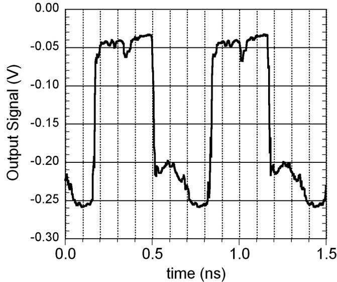
Figure 5.9: GCS divide-by-2 output waveform,  $f_{clk} = 3$  GHz,  $f_{out} = 1.5$  GHz
