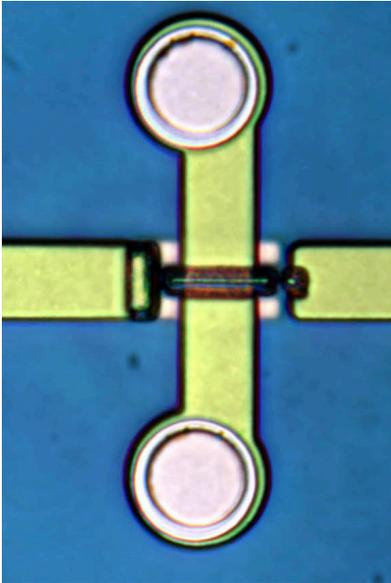
Figure 3.11: IC micrograph photo of device within test structure after passivation
