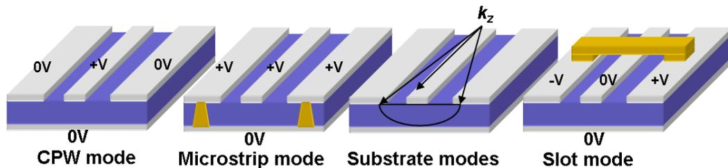
Figure 3.13: Coplanar wiring environment – showing the CPW and parasitic modes
