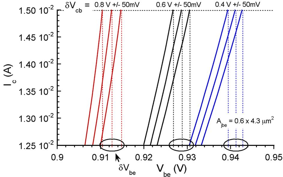
Figure 4.20: Change in  $V_{be}$  associated with differences in operating temperature for changes in  $V_{ce}$  ( $\delta V_{ce} = \delta V_{be} + \delta V_{cb}$ ), keeping  $I_c$  constant. The Gummel measurement technique is used to acquire device thermal data.
