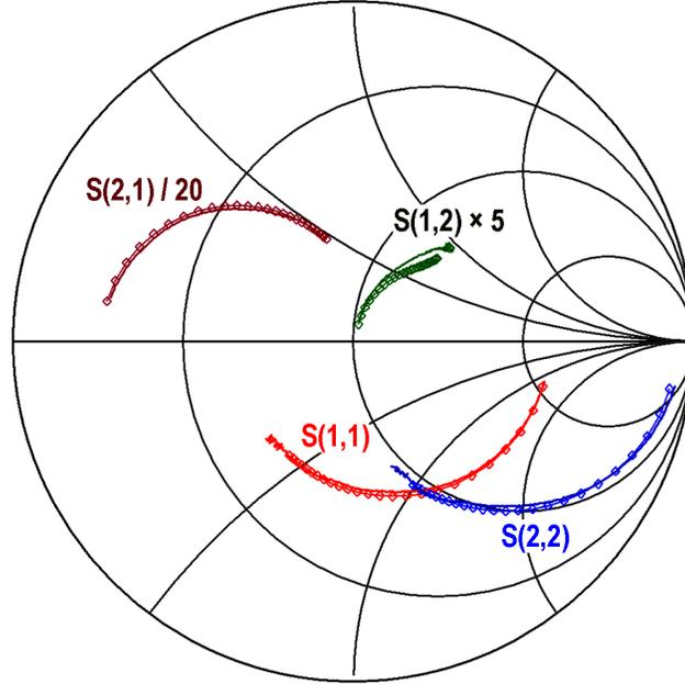
Figure 2.8: Measured (solid line) and simulated S-parameters (data points) of the HBT and hybrid- $\pi$  equivalent circuit
