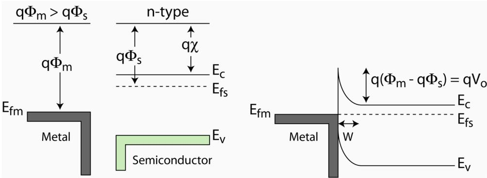
Figure A.2: Band line-up of n-type ohmic contact
