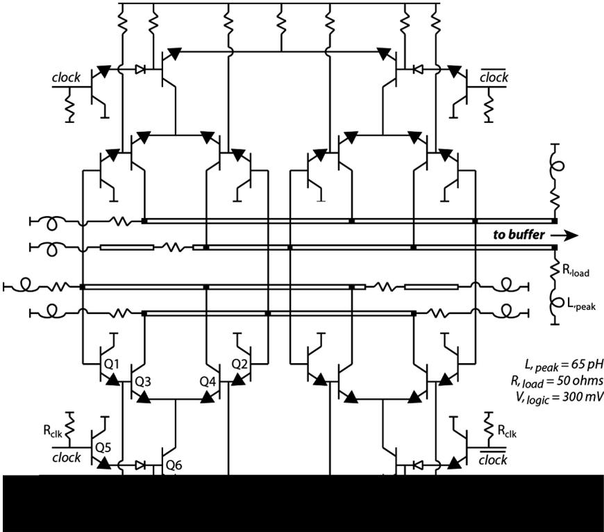
Figure 5.1: Circuit diagram of ECL static frequency divider w/ design details
