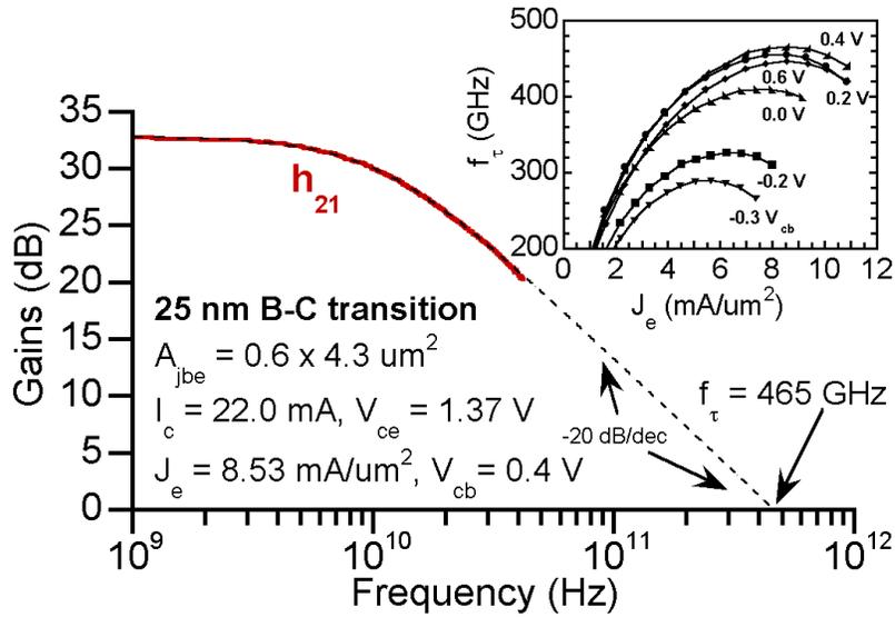
Figure 4.18: Measured microwave gains, DHBT 26 – Peak  $f_\tau$
