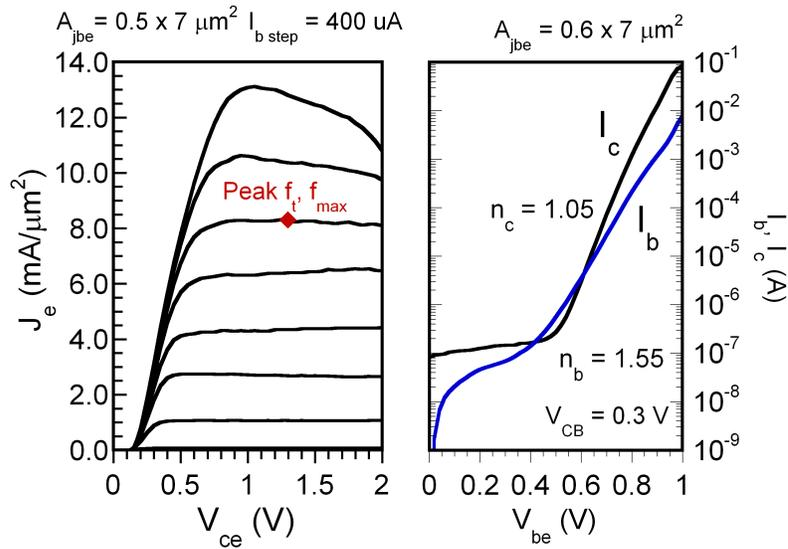
Figure 4.2: Common-emitter I-V and Gummel characteristics, DHBT 19b
