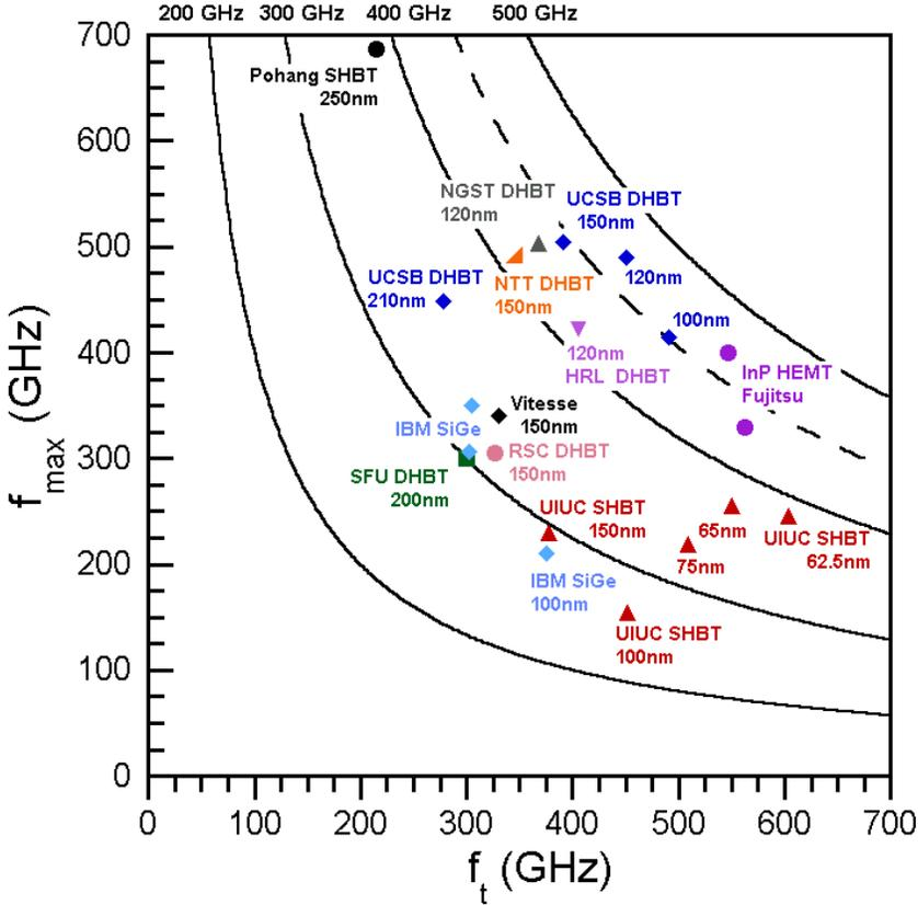
Figure 6.1: Summary of  $f_\tau$  and  $f_{max}$  performance from various HBT manufacturers at the collector thickness cited – updated June 2005
