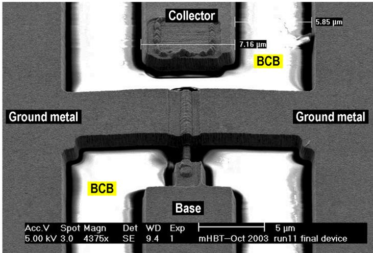
Figure 3.10: Planar device interconnect scheme: metal interconnect on 1.7 μm of BCB above InP substrate
