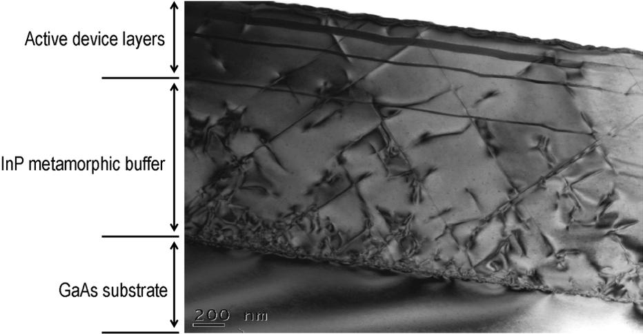
Figure 3.16: Observed InP metamorphic buffer defects from epitaxy growth
