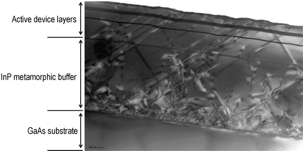
Figure 3.17: Observed InP metamorphic buffer defects—different location
