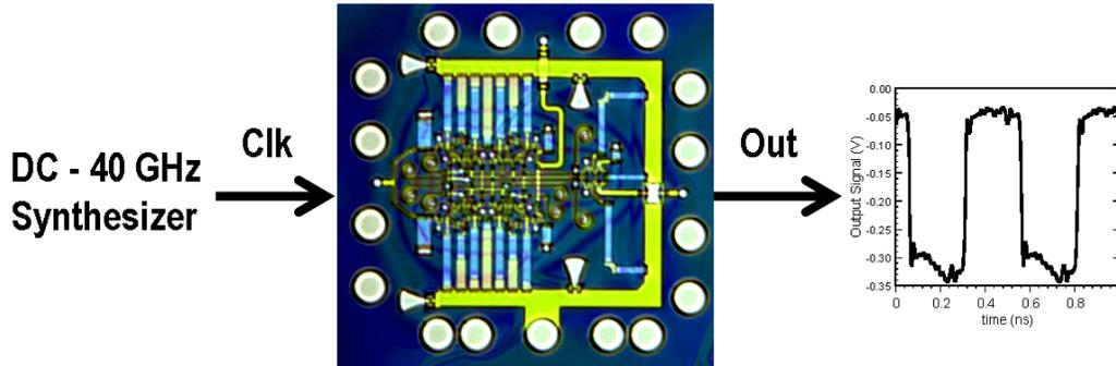
Figure 5.2: DC-40 GHz divider testing
