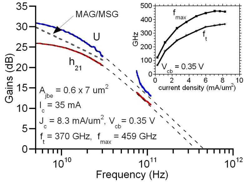
Figure 4.3: Measured microwave gains, DHBT 19b – Peak  $f_\tau, f_{max}$
