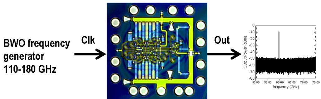
Figure 5.4: 110-136 GHz divider testing
