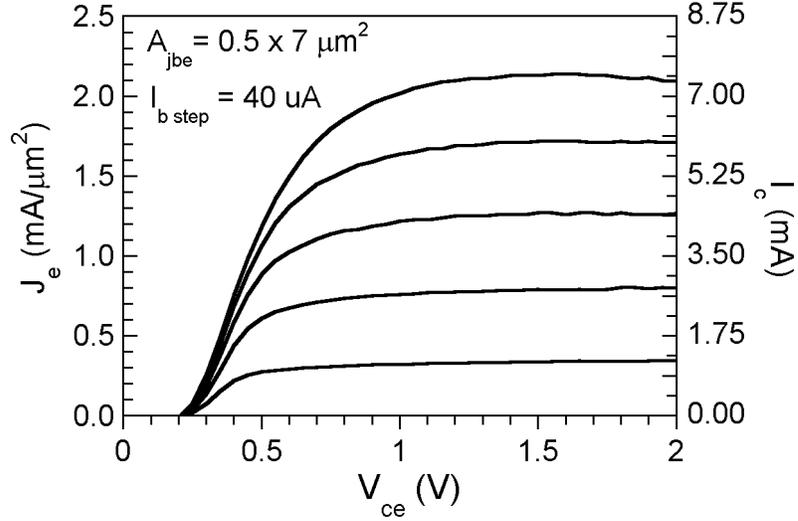
Figure 4.35: Common-emitter current-voltage characteristics, mHBT
