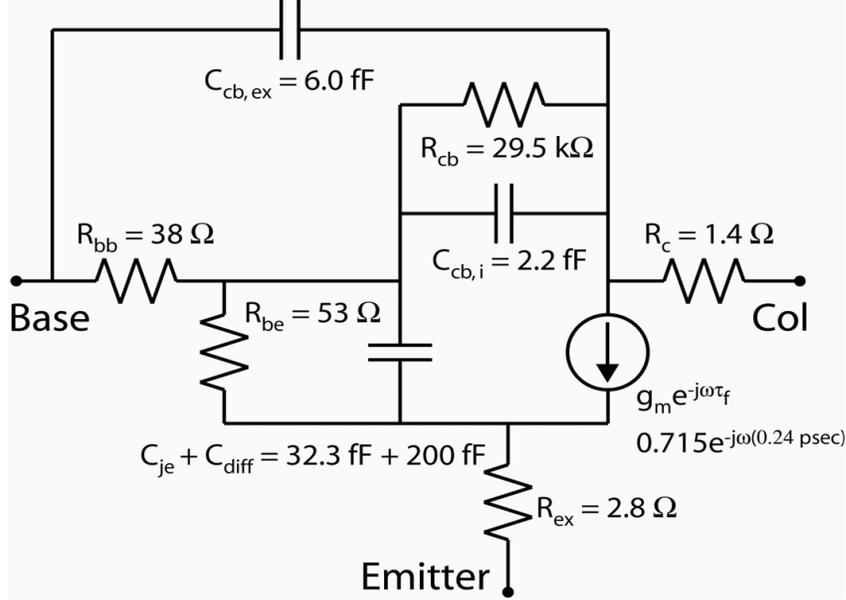
Figure 4.31: Hybrid- $\pi$  model, DHBT 27 – Peak  $f_\tau$ ,  $f_{max}$
