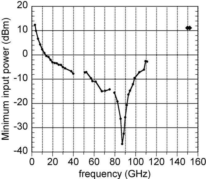
Figure 5.13: Sensitivity plot of 150 GHz divide-by-2
