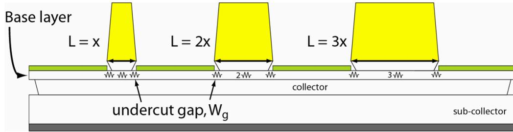
Figure 2.5: Pinned TLM structure – the emitter resides atop the base semiconductor
