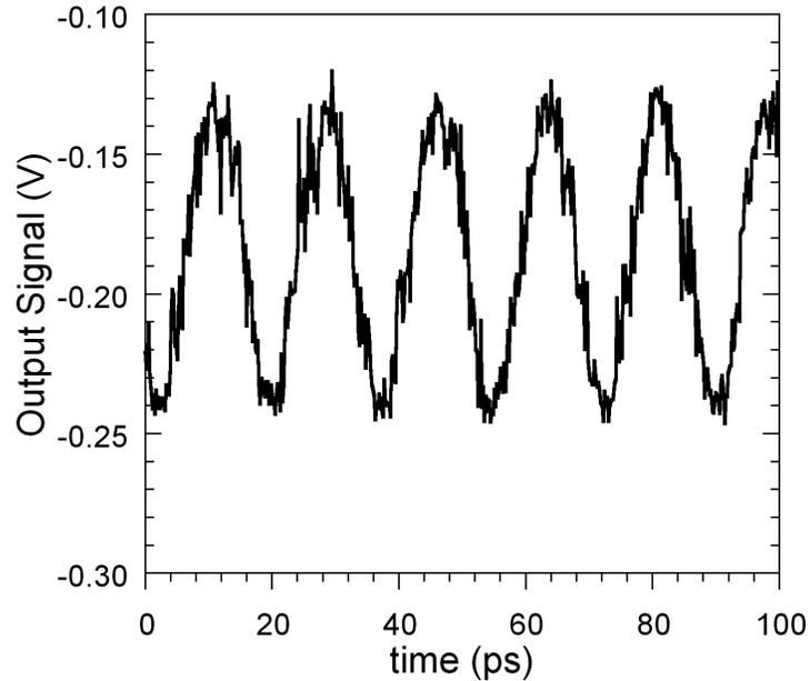
Figure 6.3: CML divide-by-2 output waveform –  $f_{clk,max} = 112.5$  GHz,  $f_{out} = 56.25$  GHz
