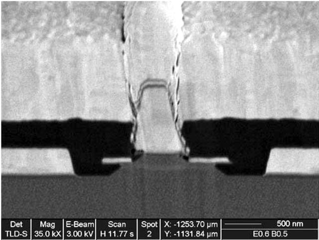
Figure 3.3: Cross-sectional SEM of an HBT after passivation and interconnect metal
