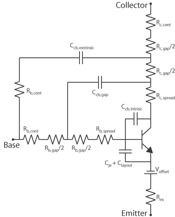
Figure 2.9: Distributed parasitics of mathematical device model
