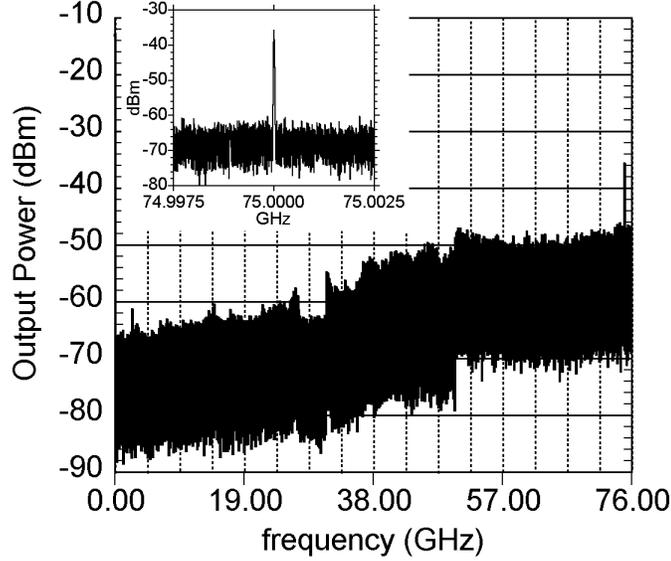
Figure 5.11: GCS fabricated divide-by-2 output spectrum,  $f_{clk} = 150$  GHz,  $f_{out} = 75$  GHz at  $T = 25^\circ\text{C}$
