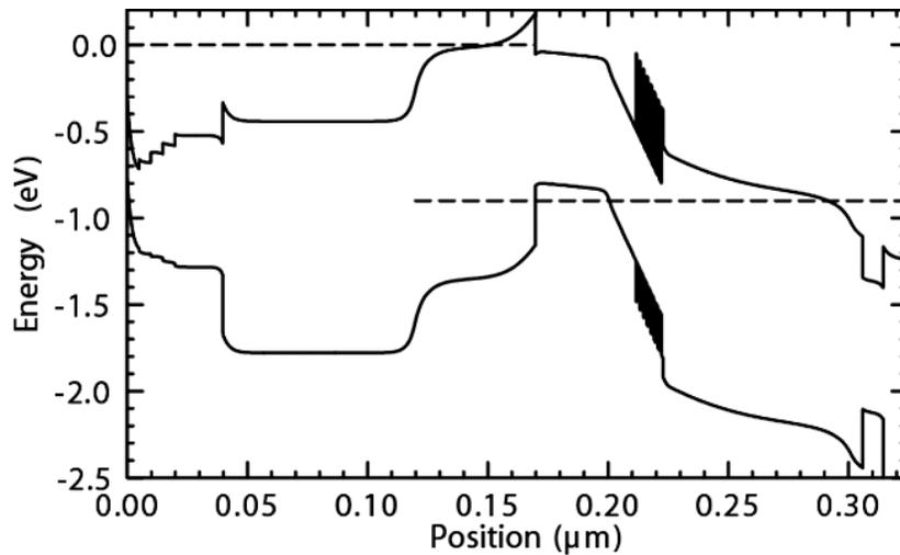
Figure 4.13: Simulated band-structure DHBT 26 –  $V_{be} = 0.9$  V,  $V_{cb} = 0.0$  V
