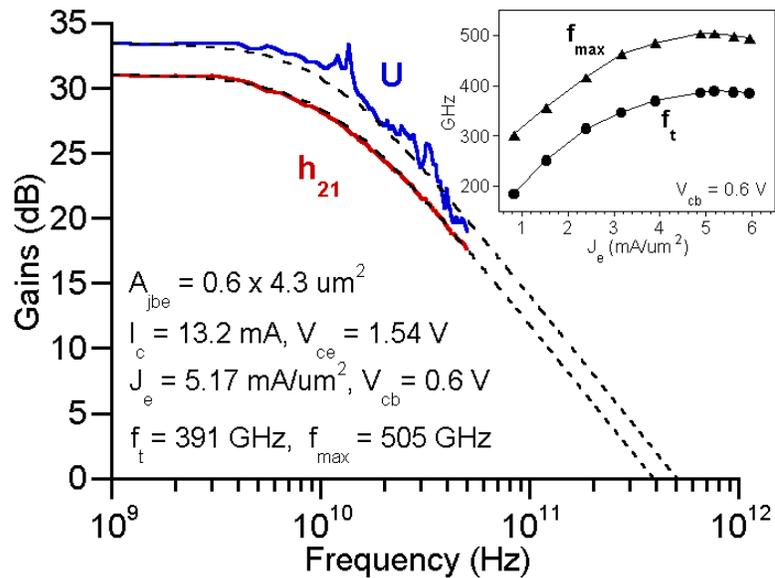
Figure 4.6: Measured microwave gains, DHBT 22 – Peak  $f_\tau$ ,  $f_{max}$
