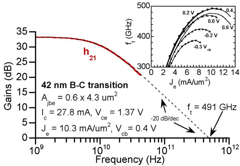
Figure 4.16: Measured microwave gains, DHBT 25 – Peak  $f_t$
