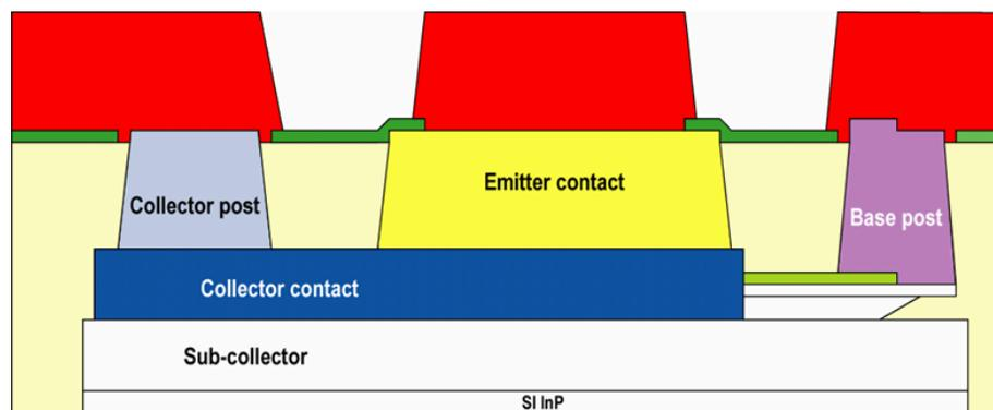
Figure 3.7: Updated HBT cross-section after passivation and Metal-1 interconnect
