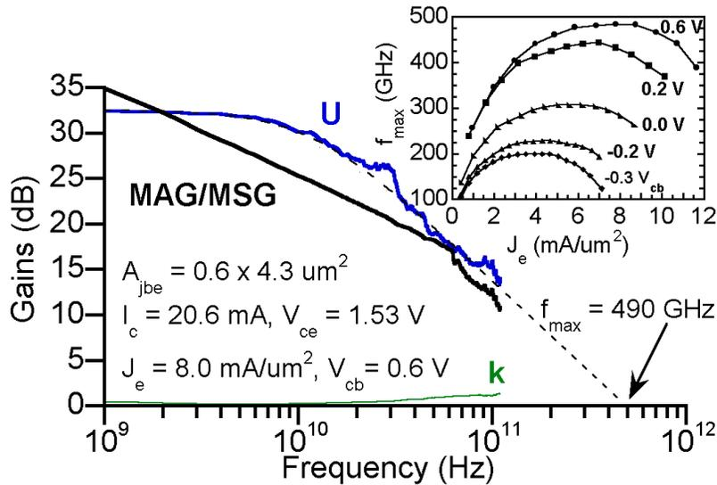
Figure 4.30: Measured microwave gains, DHBT 27 – Peak  $f_{max}$
