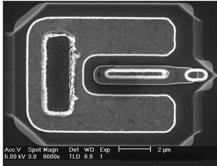
Figure 3.8: SEM, top view – 0.6  $\mu\text{m}$  emitter width, 1.3  $\mu\text{m}$  collector mesa width
