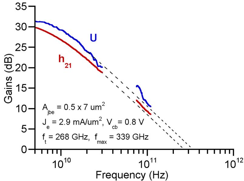
Figure 4.37: Measured microwave gains for 200 nm collector metamorphic DHBT – Peak  $f_t$ ,  $f_{max}$
