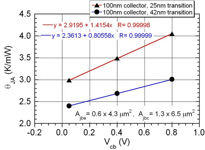
Figure 4.21: Variance of thermal resistance  $\theta_{JA}$  with changing collector potential  $V_{cb}$
