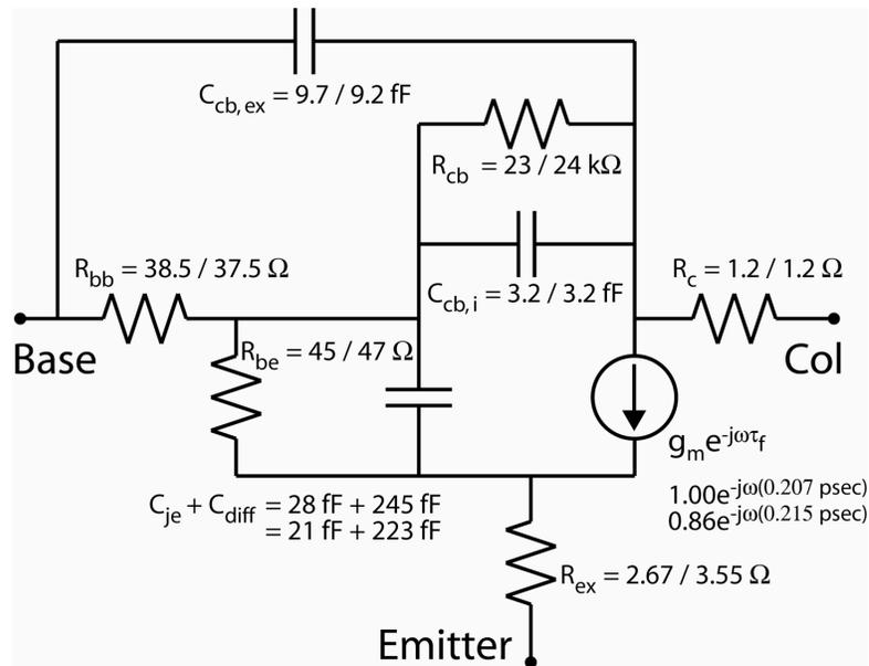
Figure 4.23: Hybrid- $\pi$  models, 100 collector, 42 / 25 nm transitions – Peak  $f_\tau$ ,  $f_{max}$
