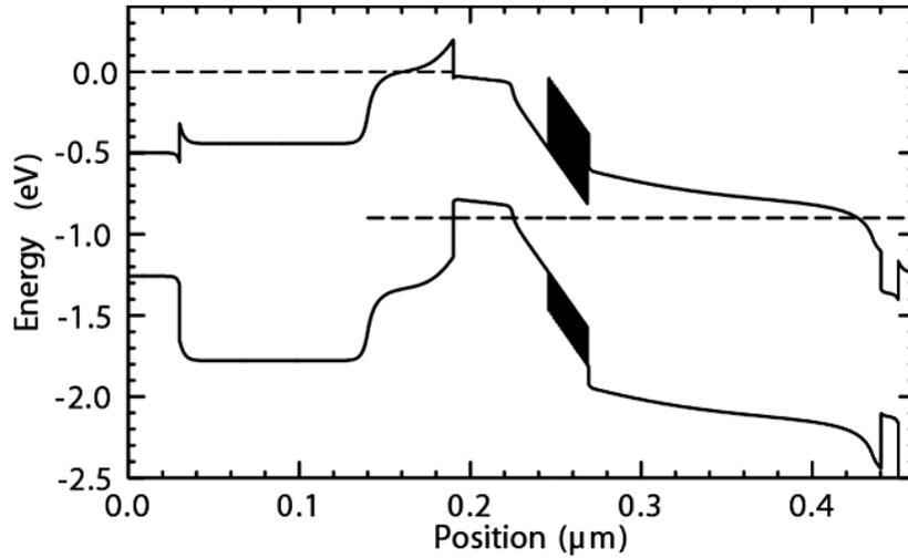
Figure 4.8: Simulated band-structure DHBT 24 –  $V_{be} = 0.9$  V,  $V_{cb} = 0.0$  V
