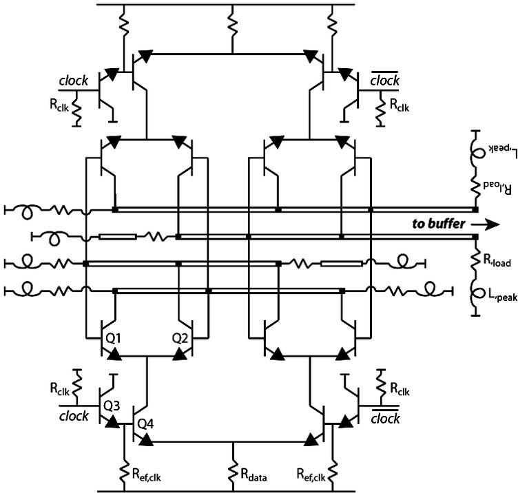
Figure 6.2: Circuit diagram of current mode logic (CML) static frequency divider
