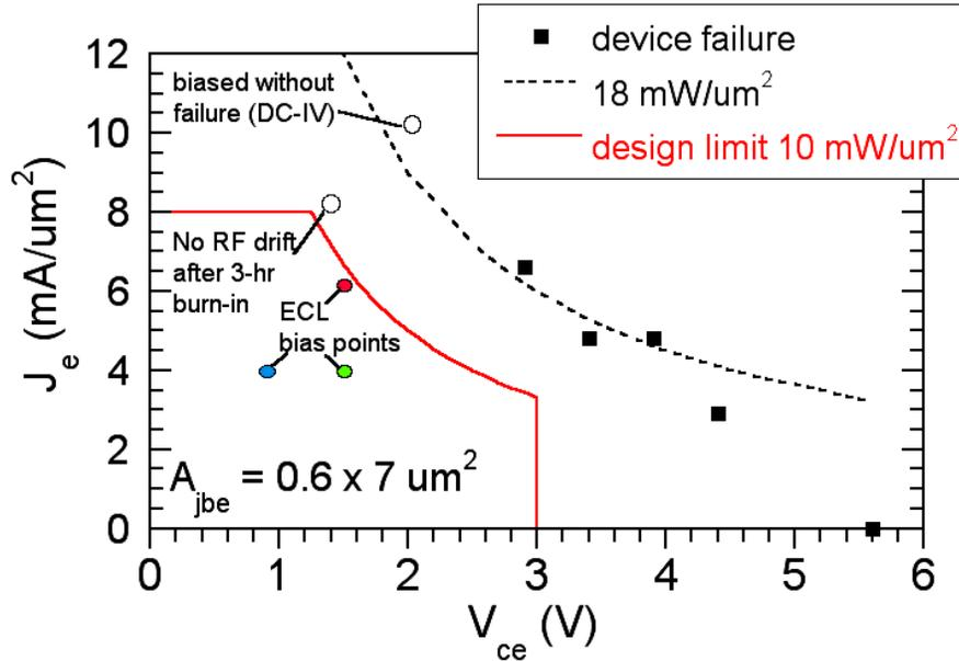
Figure 2.10: InP DHBT safe operating area plot – 150 nm collector, 30 nm base
