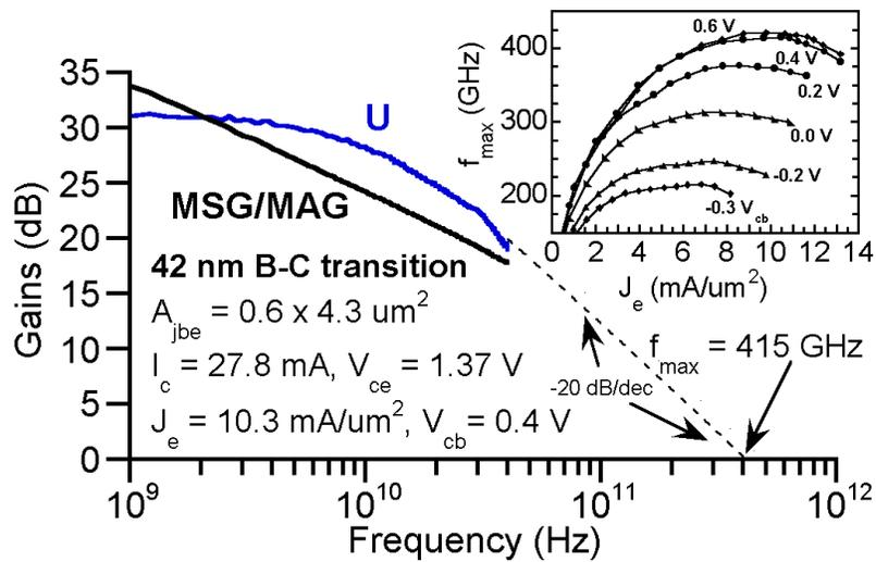
Figure 4.17: Measured microwave gains, DHBT 25 – Peak  $f_{max}$
