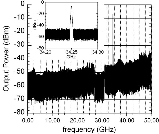
Figure 5.10: GCS fabricated divide-by-4 output spectrum,  $f_{clk} = 137$  GHz,  $f_{out} = 34.25$  GHz
