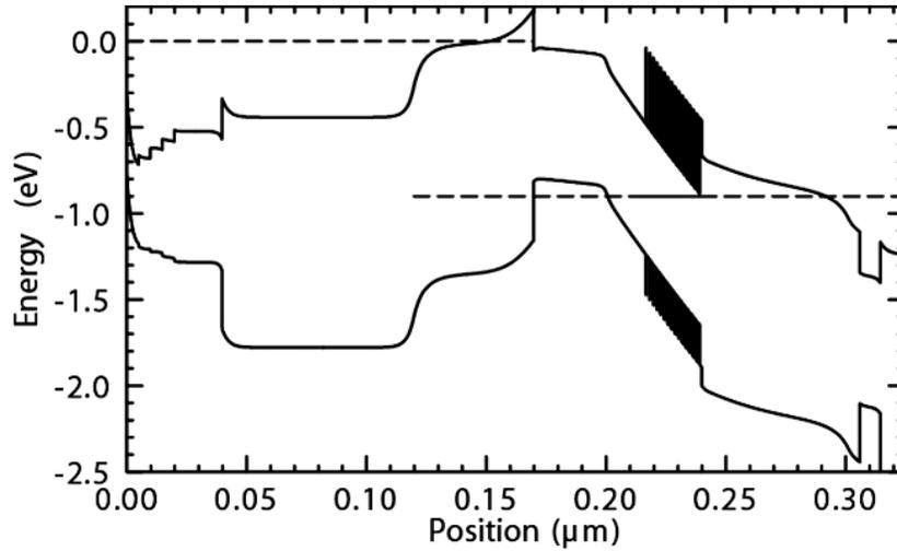
Figure 4.12: Simulated band-structure DHBT 25 –  $V_{be} = 0.9$  V,  $V_{cb} = 0.0$  V
