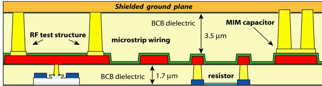
Figure 3.14: Cross-section of the mesa HBT process, showing its thin-film microstrip wiring environment
