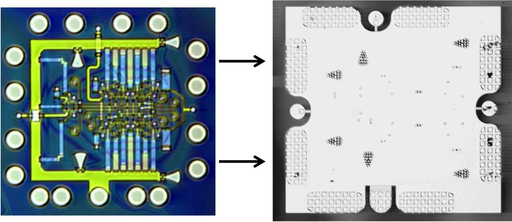
Figure 3.15: Fabricated divide-by-2 before and after final ground-plane metalization
