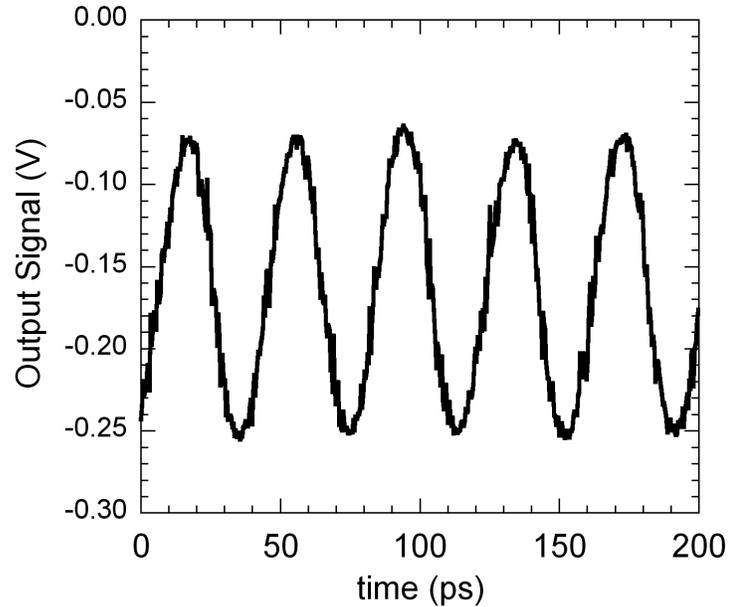
Figure 6.4: Ultra low power CML divide-by-2 output waveform –  $f_{clk,max} = 51$  GHz,  $f_{out} = 25.5$  GHz
