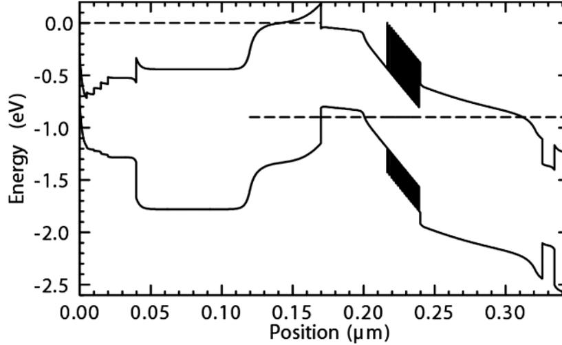
Figure 4.25: Simulated band-structure DHBT 27 –  $V_{be} = 0.9$  V,  $V_{cb} = 0.0$  V
