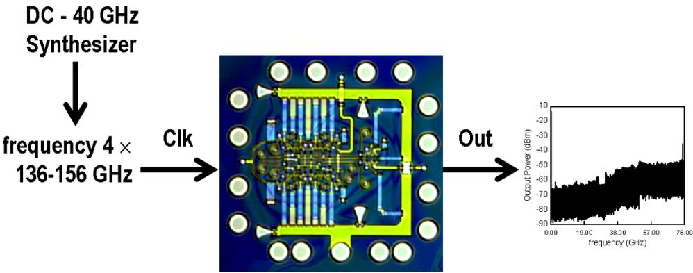
Figure 5.5: 136-156 GHz divider testing
