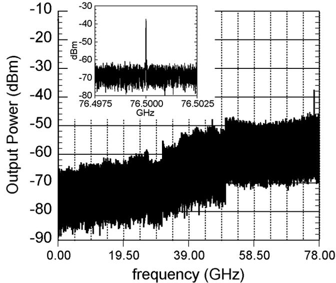
Figure 5.12: GCS fabricated divide-by-2 output spectrum,  $f_{clk} = 153$  GHz,  $f_{out} = 76.5$  GHz at  $T = 20^\circ\text{C}$
