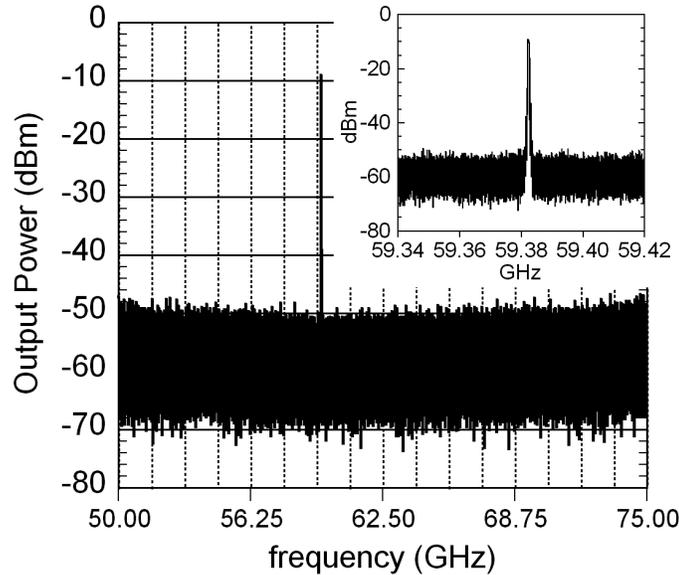
Figure 5.6: GCS fabricated divide-by-2 output spectrum,  $f_{clk} = 118.70$  GHz,  $f_{out} = 59.35$  GHz
