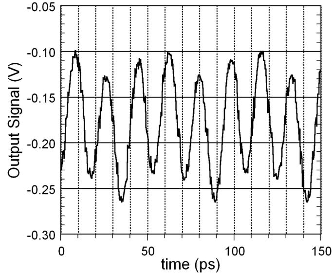
Figure 5.15: UCSB divide-by-2 output waveform,  $f_{clk} = 113.1$  GHz,  $f_{out} = 56.55$  GHz—the highest available sampling scope measurement
