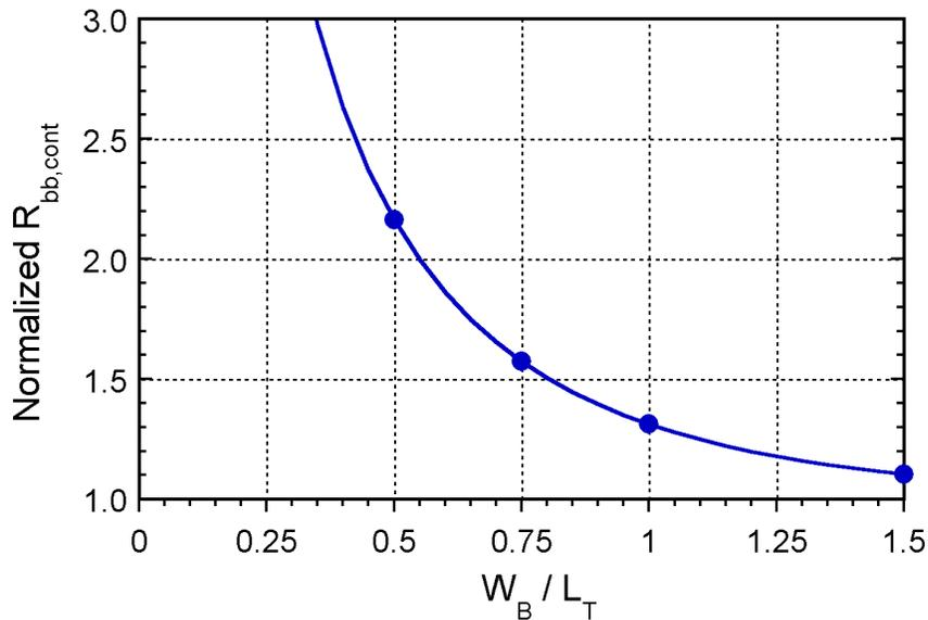
Figure 2.14: Variance of the contact resistance (normalized to  $\frac{\sqrt{\rho_c \rho_c}}{2L_e}$ ) as the base contact is scaled
