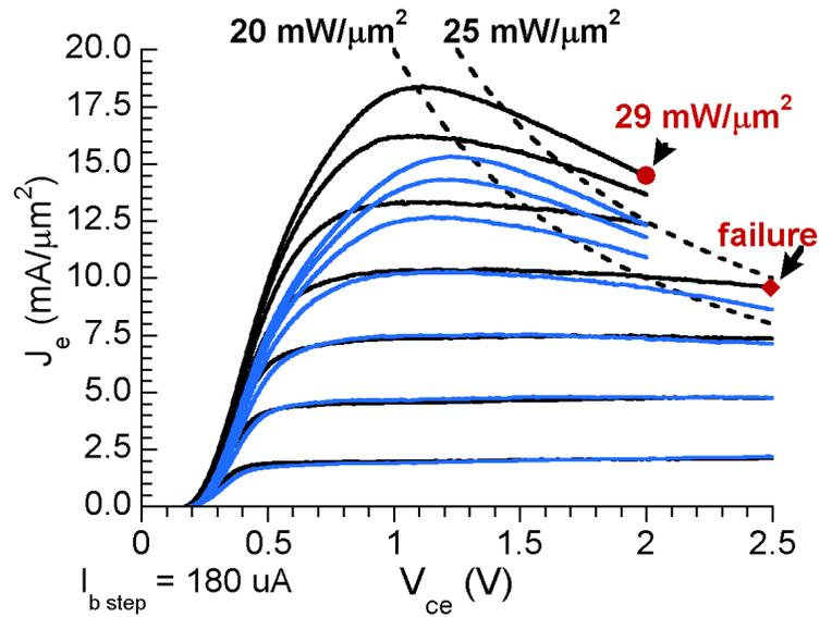
Figure 4.22: High-power density common-emitter curves – 42 nm transition (DHBT 25) black, 25 nm transition (DHBT 26) blue
