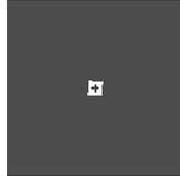
The center of the Tr mark is the center of the TIS mark, and indicates the position of the mark on the reticle.
