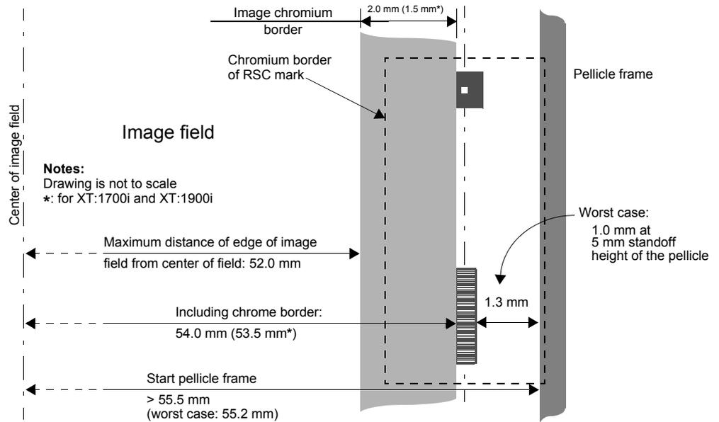
Figure 4.8 Enlarged view of placement of one of the vertical marks
