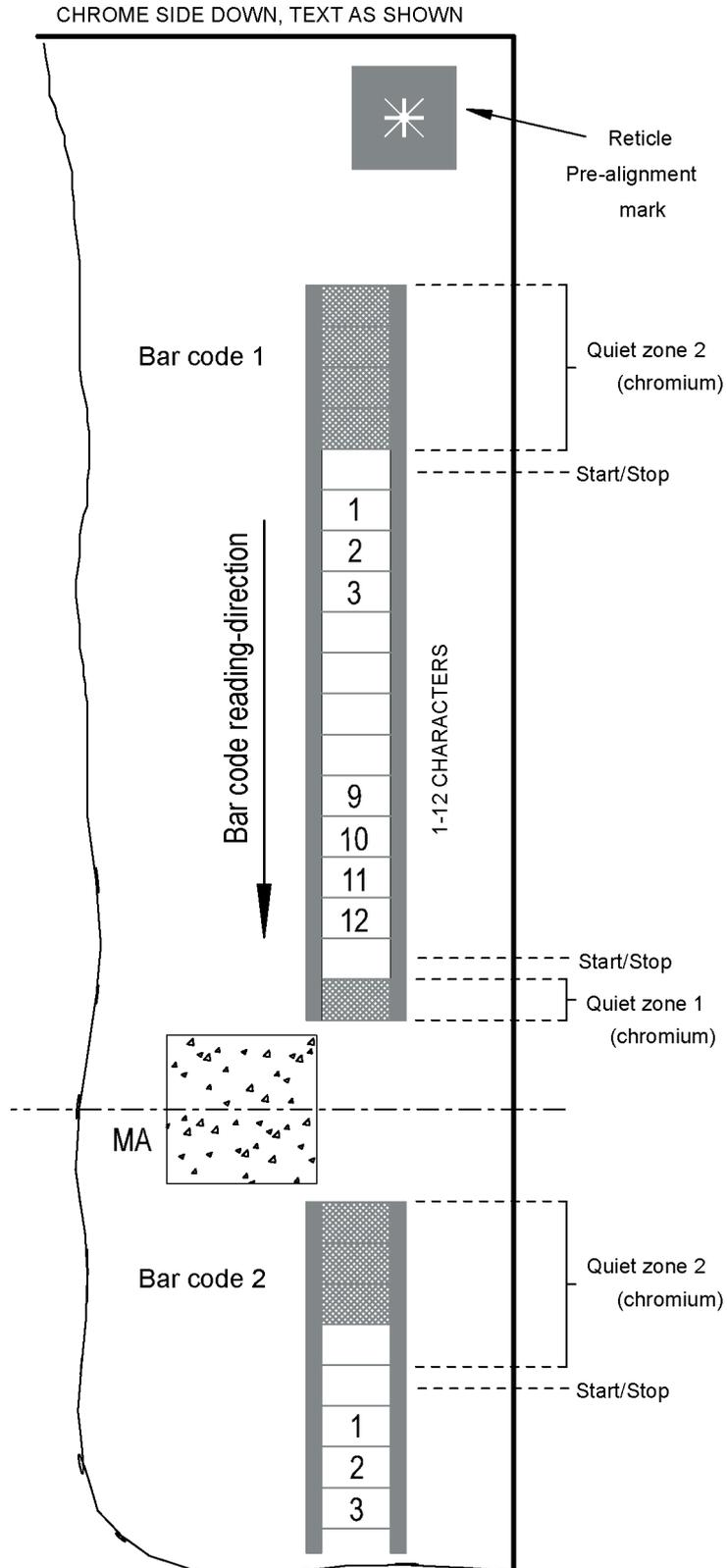
Figure 3.13 The orientation of the Bar Code on the reticle
