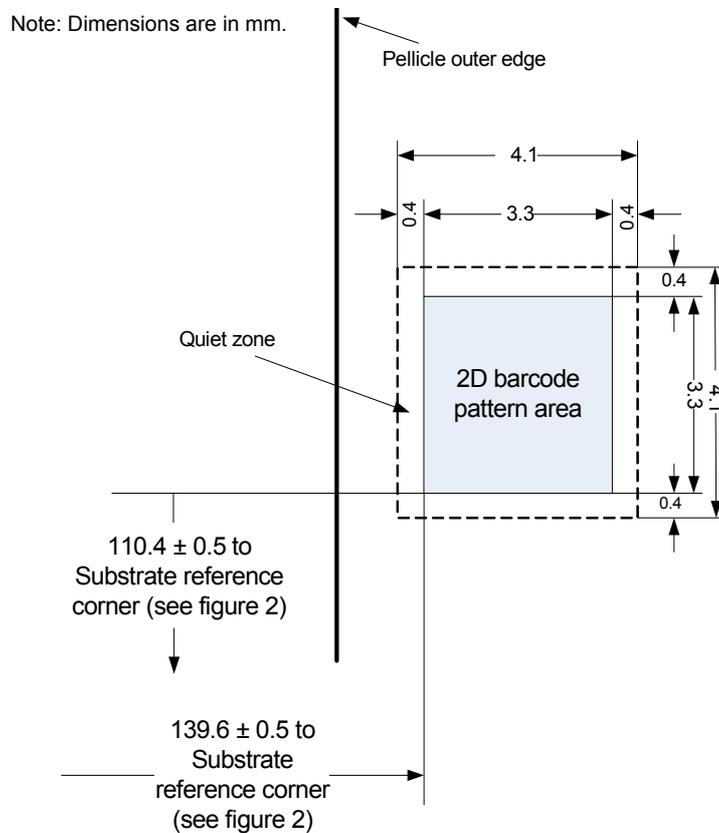
Figure 3.19 Details of location 'B' (right)
