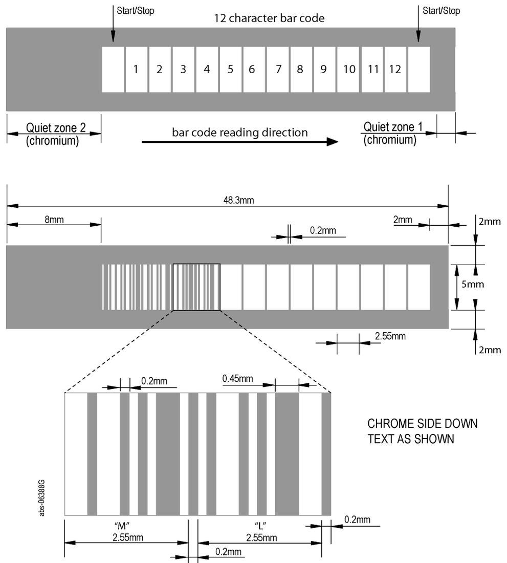
**Figure 3.14** The bar code structure and dimensions
