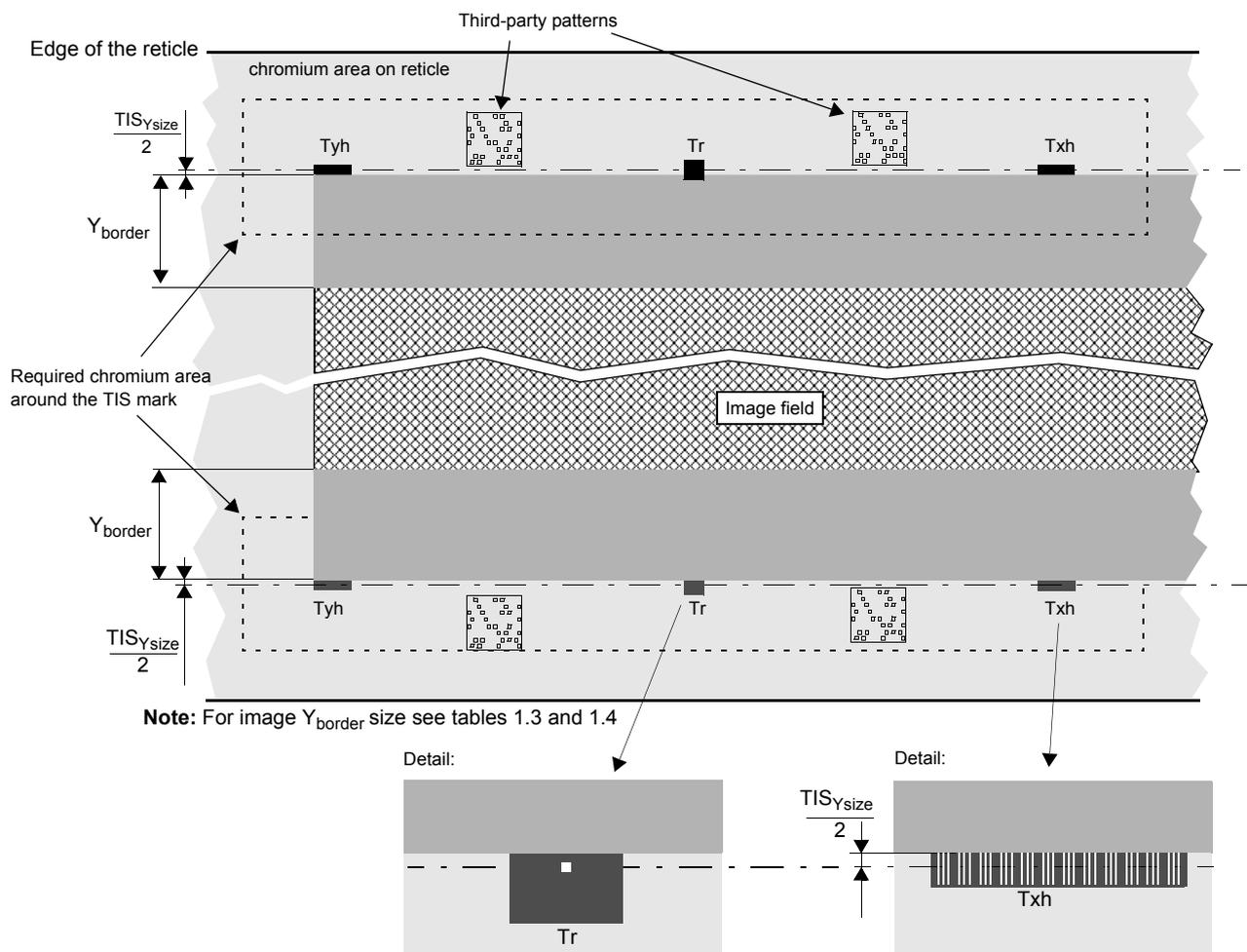
Figure 3.6 Example of the use of various chromium borders (Y direction)
