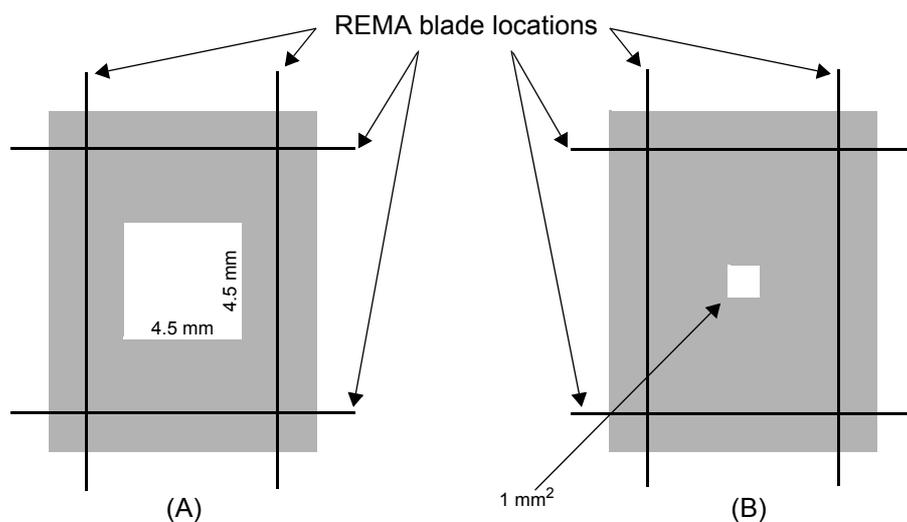
Figure 3.11 Example of a normal and extended image border (scanner situation)
