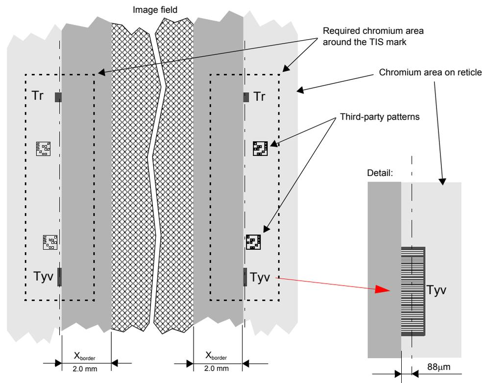
Figure 3.7 Example of various chromium borders (X direction) with TIS\_RSC-marks on the left and right side of the image field
