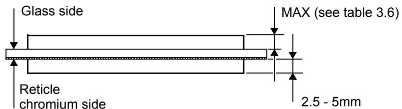
**Figure 3.21** Pellicle frame standoff height
