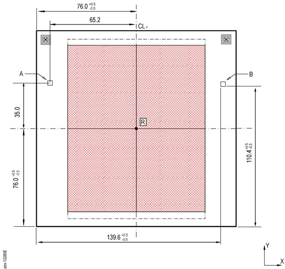
**Figure 3.17** The two supported locations for a 2D bar code
