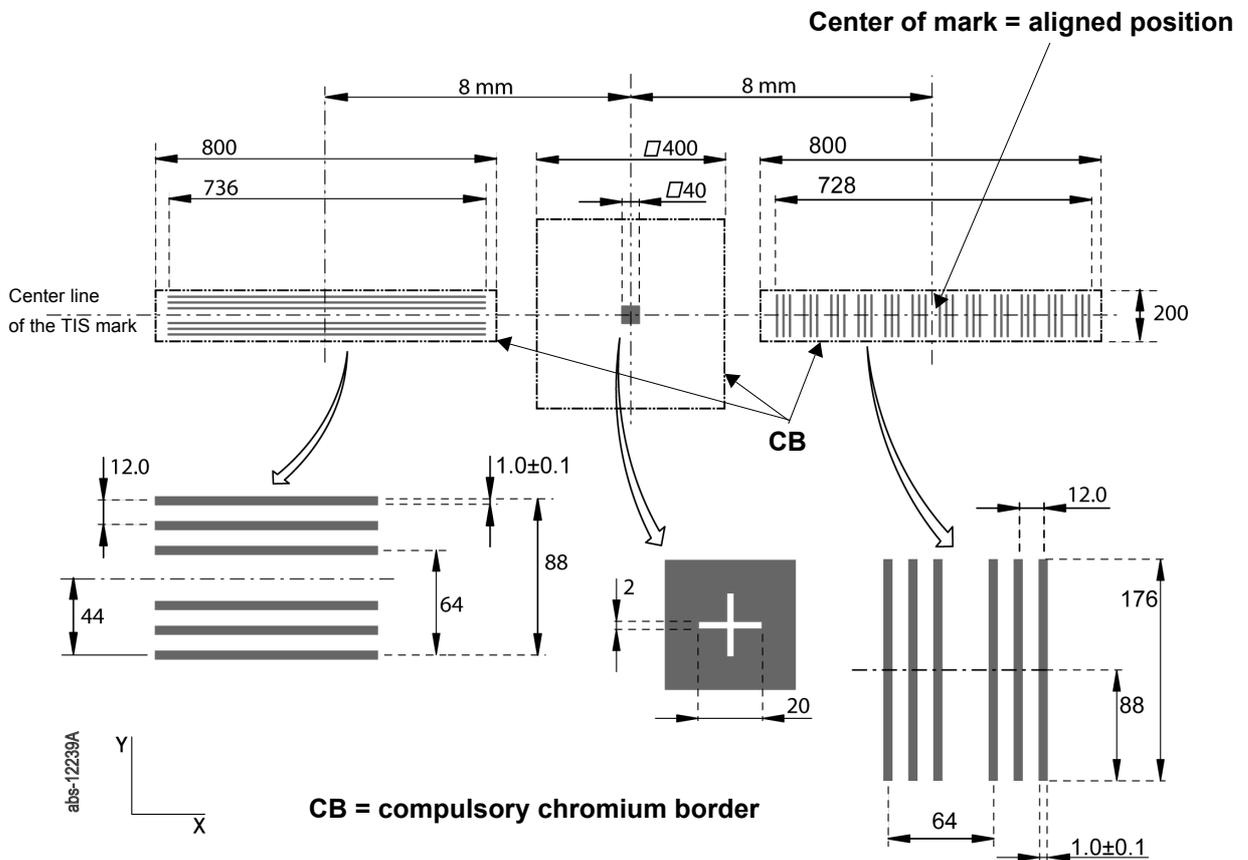
Figure 3.4 Dimensions of the standard TIS\_RBA-mark
