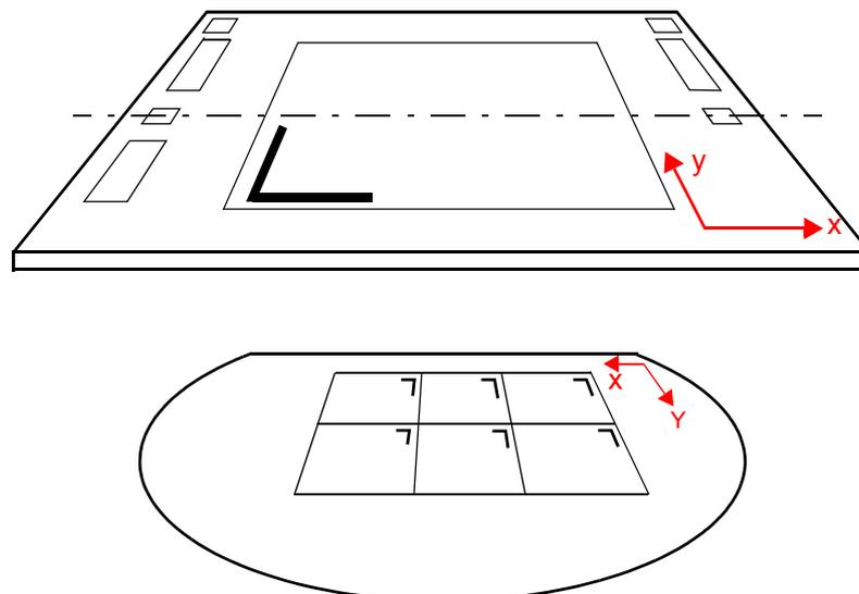
**Figure 5.1** Relationship between reticle and wafer coordinate system
