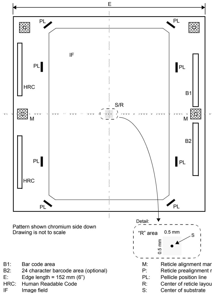
Figure 5.2 Schematic layout of a PAS 5500 5X (6 inch) reticle
