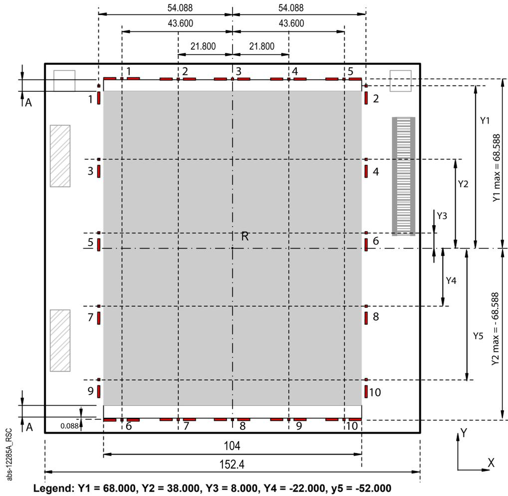
Figure 4.9 Default mark layout for RSC marks
