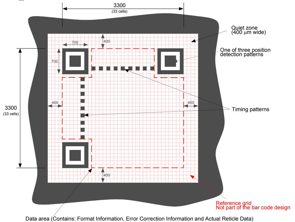
**Figure 3.15** The basic 2D Barcode field (without data)
