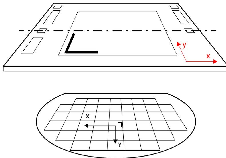
Figure 1.2 Relationship between reticle and wafer coordinate system
