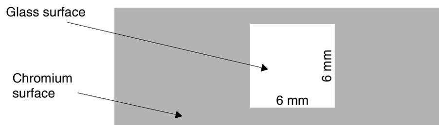
Figure 3.20 Release pin area
