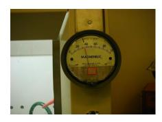
\*"Magnihelic gauge" – note normal gauge position. Significant deviation may indicate condition low air flow.
