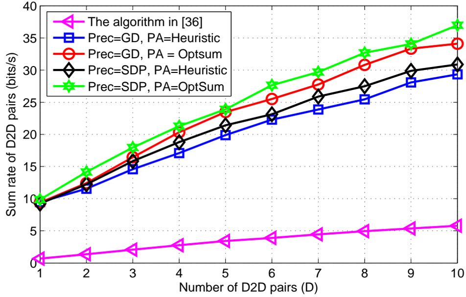
Figure 6.1: Effect of number of D2D pairs on the achievable sum of D2D rates for different combinations of precoding and PA techniques.
