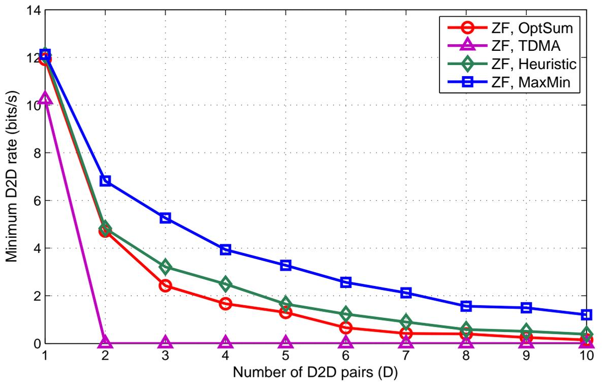
Figure 4.4: Effect of number of D2D pairs on the minimum of D2D rates for different PA techniques.
