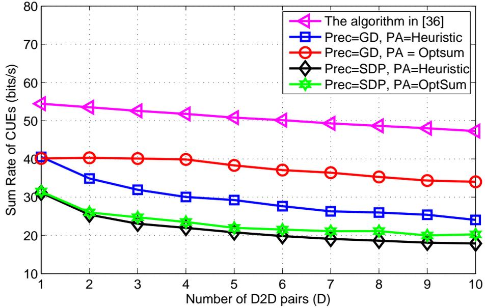
Figure 6.2: Effect of number of D2D pairs on the achievable sum of D2D rates for different combinations of precoding and PA techniques.
