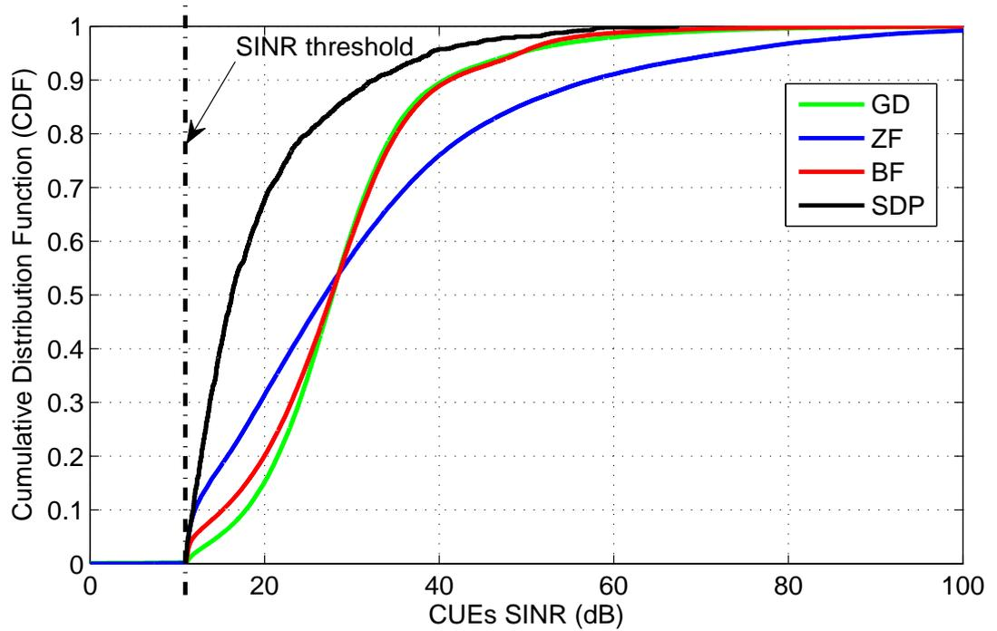
Figure 5.3: CDF of the SINR of the CUEs under different precoding techniques.  $N = 100, D = 3$ .
