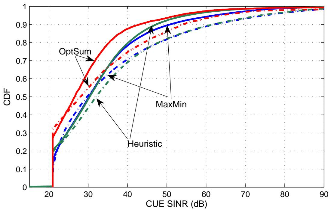
Figure 4.6: CDF of the SINR of the CUEs under different PA and precoding techniques. Solid lines represent ZF precoder. Dashed lines represent BF precoder.  $D = 3$ .
