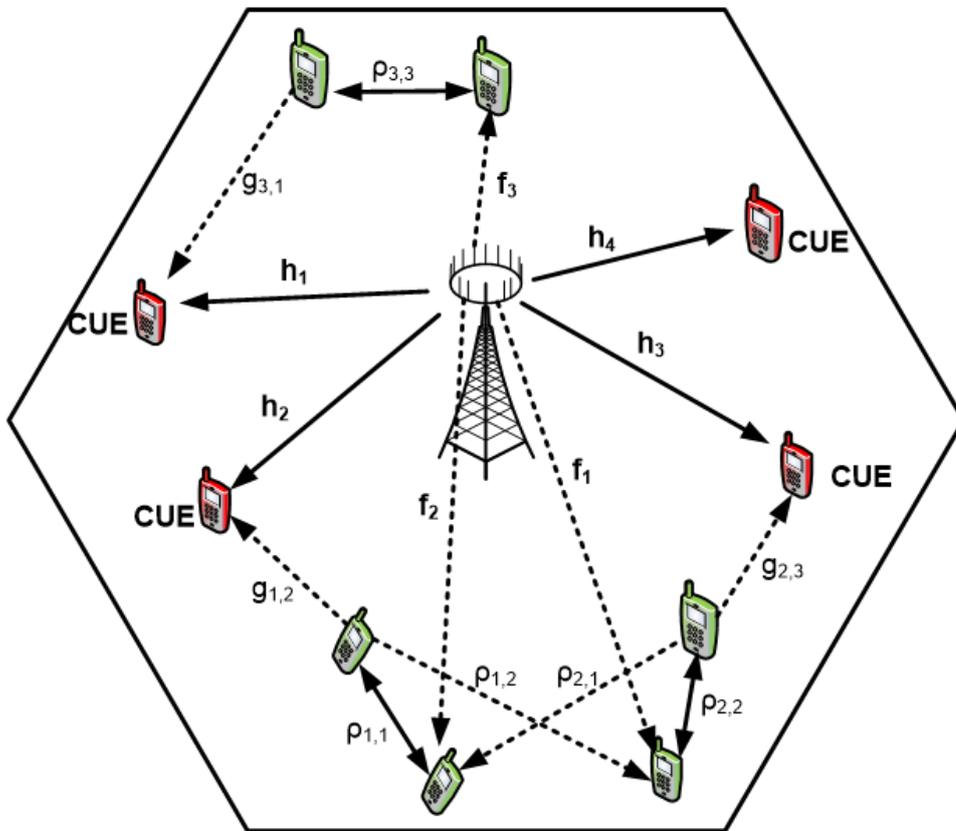
Figure 3.1: Single cell multicasting network with Massive MIMO,  $K = 4$  cellular users (red terminals),  $D = 3$  D2D pairs (green terminals). Dashed lines represent interference.
