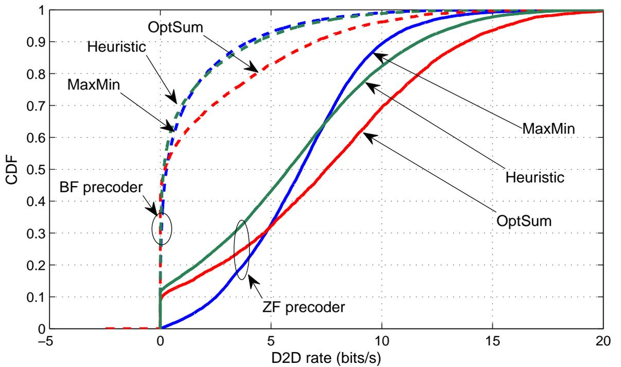
Figure 4.5: CDF of the D2D achievable rates under different PA and precoding schemes.  $D = 3$ .
