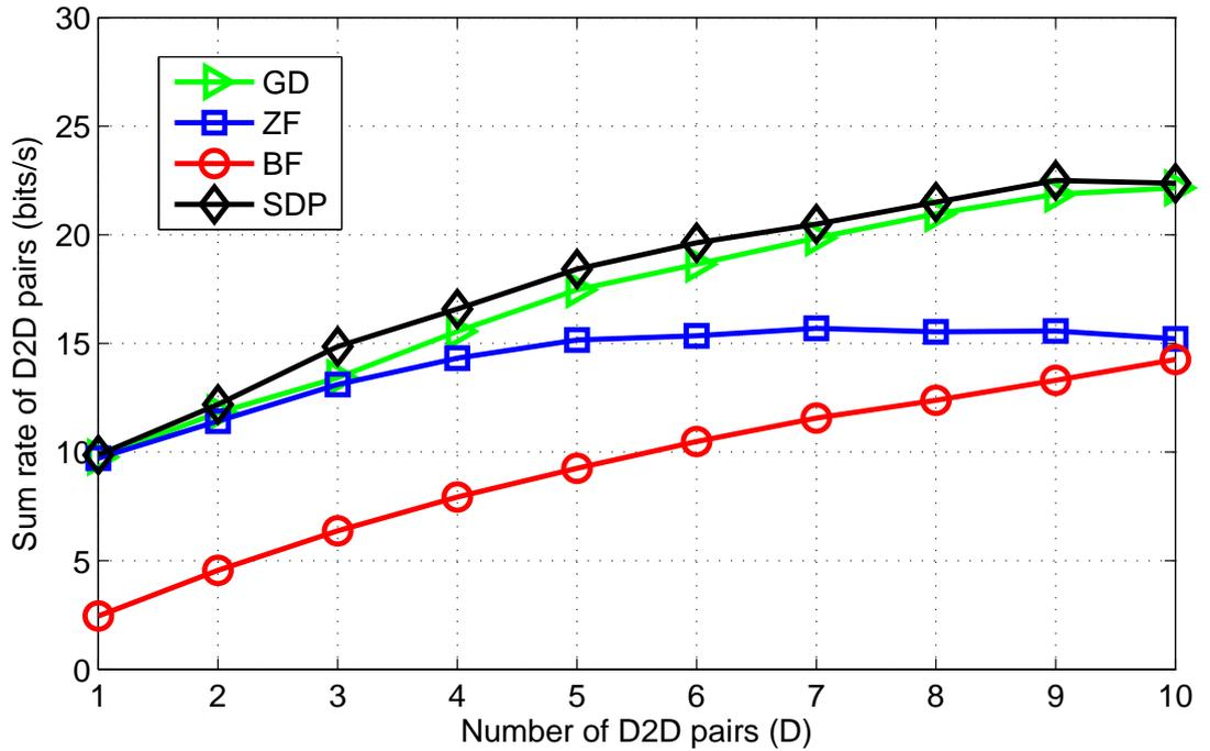
Figure 5.1: Effect of the number of D2D pairs on the performance of different precoding schemes.  $N = 100$ .
