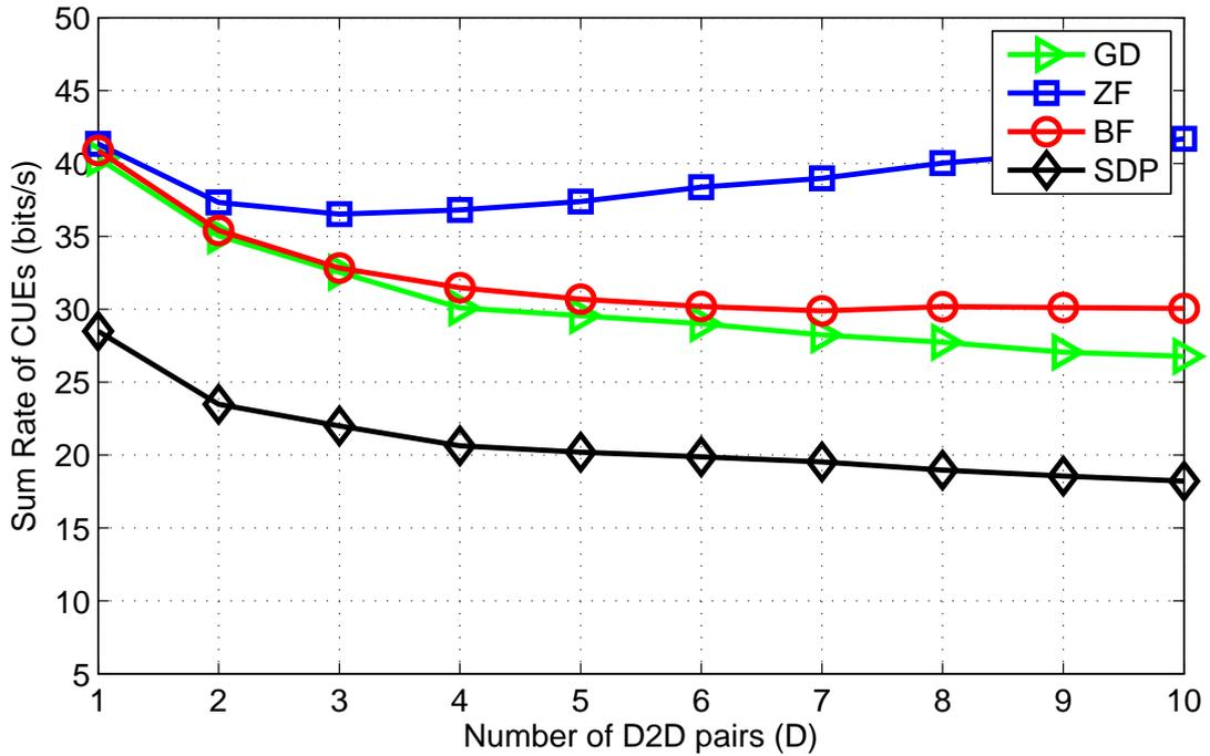
Figure 5.2: Effect of number of D2D pairs on the achievable sum of CUE rates for different precoding techniques.  $N = 100$
