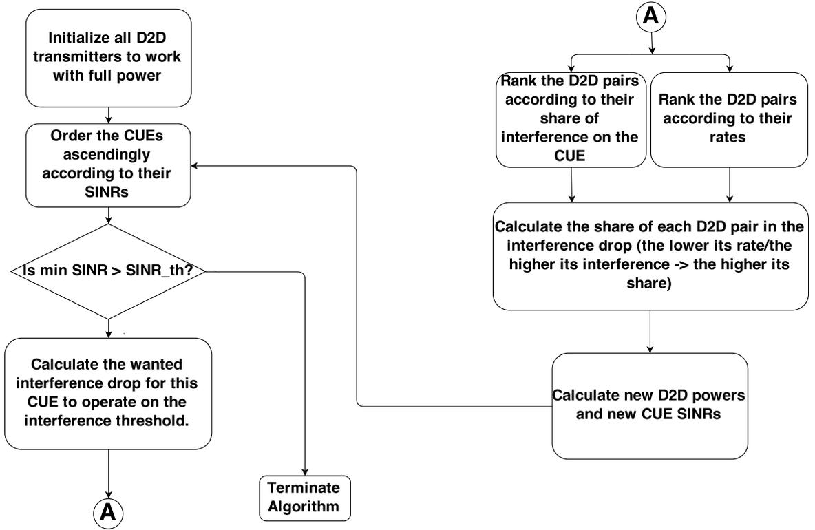
Figure 4.1: Flowchart of the Heuristic PA algorithm
