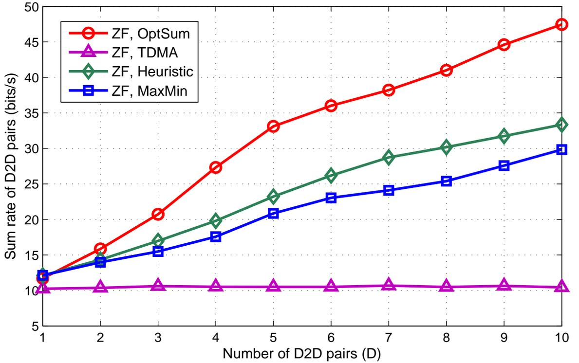
Figure 4.3: Effect of number of D2D pairs on the achievable sum of D2D rates for different PA techniques.
