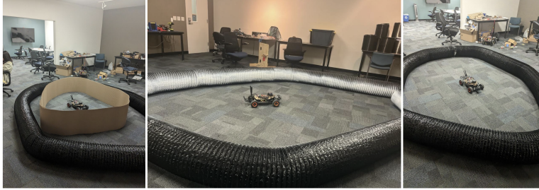
Figure 5: Test setup for LiDAR skipping on various track materials.
