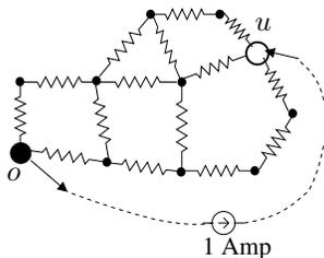
Figure 1: A resistive electrical network for which a 1 Ampere current was injected at node  $u$  and extracted at the reference node  $o$ . The resulting potential difference  $V_u - V_o$  is the effective resistance between  $u$  and  $o$ .
