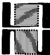
d. 2-Element rosette 90^\circ planar foil strain gage
