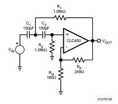
$$\frac{V_{OUT}}{V_{IN}} = \frac{K_0 s^2}{s^2 + s \left(\frac{1}{R_2} \left(\frac{1}{C_1} + \frac{1}{C_2}\right) + \frac{1 - K_0}{R_1 C_1}\right) + \frac{1}{R_1 R_2 C_1 C_2}}$$
