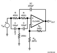
$$\frac{V_{OUT}}{V_{IN}} = \frac{K_0 \left(s^2 + \frac{1}{R^2 C^2}\right)}{s^2 + 2\frac{s}{RC} \left(2 - K_0\right) + \frac{1}{R^2 C^2}}$$
