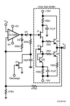
50ns pulses over a 20mV to 1.5V input range.
