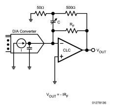
For example, with the CLC401,  $R_F = 2.5k\Omega$  and a D/A output capacitance of 20pF, C  $\cong$  5pF.
