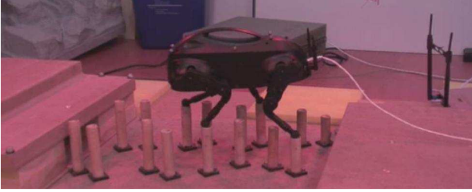
Fig. 1. LittleDog walks carefully on pegs
