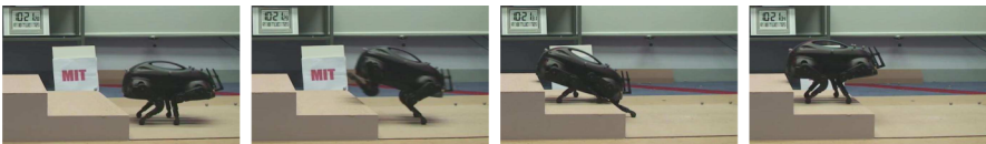
Fig. 2. LittleDog climbs a step dynamically
