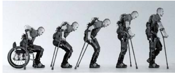
Figure 1.7: The exoskeletons have shown the ability to restore mobility to those confined to wheelchairs. The Ekso Bionic E-legs shown above have a mass of 20 kg and have a top speed of 0.9 m/s. As can be seen by the added mass studies in Section 4.2, this mass is a substantial and non-negligible load on the user and/or exoskeleton.
