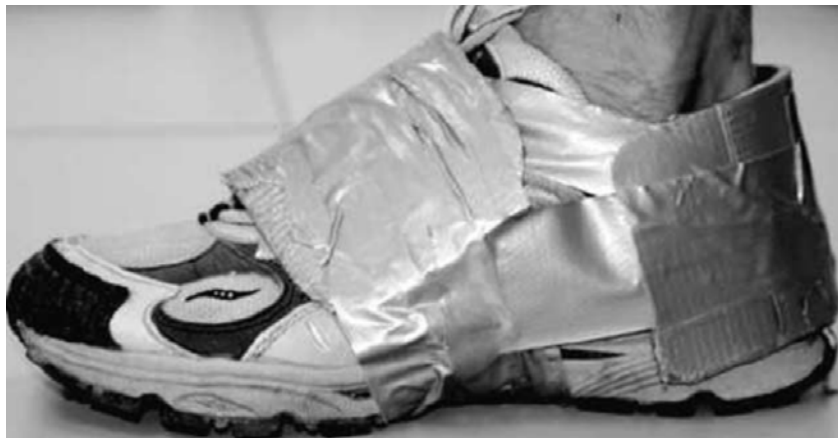
Figure 4.13: This figure depicts the mass placement for Browning et al. [45]. Note that the lead weights were placed on the shoelaces as well as on the heel of the shoe. The added mass study presented here utilized therapy weights (vinyl covered bags filled with steel pellets). Due to the higher volume of steel pellets, the weight was fastened to the shoelace section of the shoe with tape.
