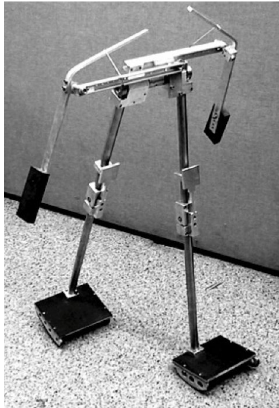
Figure 1.3: This walking robot designed by Collins et al. [1] utilized passive dynamics for stabilization and locomotion. The energy lost through impact is made up for by the robot's walking on a slight decline. This robot builds on the work of McGeer, who built a passive walker with knees, designed with an inner and an outer pair of legs, to prevent motion in the frontal plane and constrain passive walking to an essentially 2D dynamic process, in the sagittal plane [2]. The Collins walker [1] shown above builds on that work, but uses curved feet that enable rocking, side-to-side motions to occur in sync with the forward motion of walking, and uses the arm momentum for yaw stabilization.
