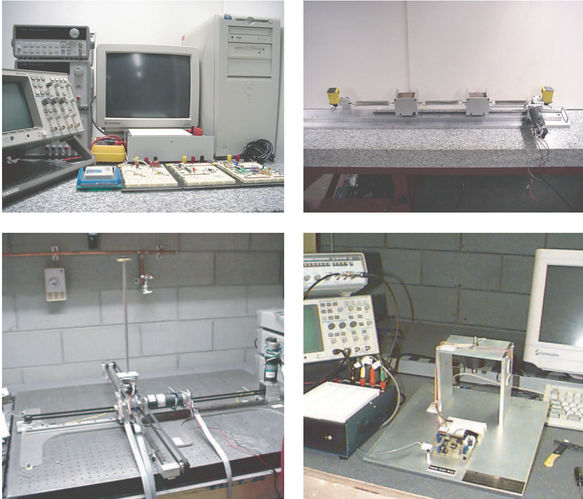
Figure 2-33: RPI mechatronics teaching lab hardware. At top, left each station is equipped with a 'scope, function generator, multi-meter, powered protoboard and a PC (with a dSPACE controller board and MATLAB/Simulink to implement real-time control). Top right: A two-mass, three-spring system demonstrates free and forced vibrations, colocated and non-colocated control, and principles of dynamic vibration absorption. The hardware includes two DC motors (with tachs), optical encoder, and two infrared position sensors. The lower left picture shows an inverted pendulum that is mounted with a universal joint and actuated through two belt-driven linear slides. The system is controlled in dSPACE using full state LQR feedback. In the final project shown, a 1/2-inch steel ball is magnetically levitated using an analog lead controller (to command current). Light from an infrared diode emitter is detected with a phototransistor. Images were obtained from the RPI Mechatronics website [51].
