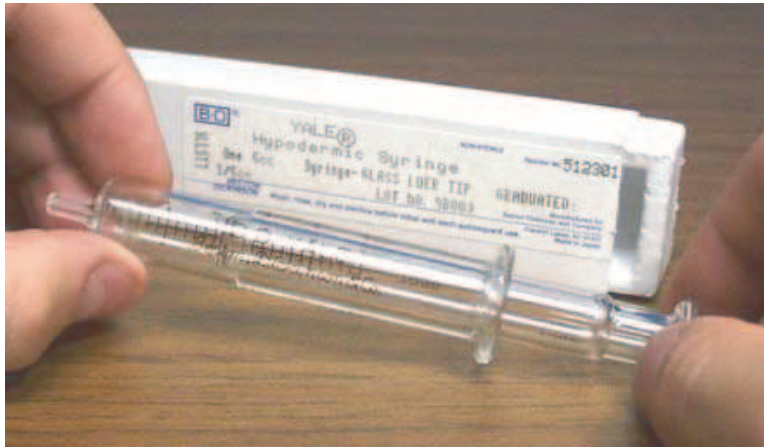
Figure 4-27: Viscous damping of thin oil layer between syringe walls
