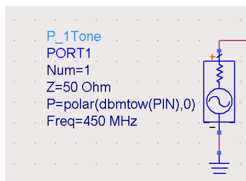
Figure 2. Single frequency source. Frequency, source impedance, and available power must be specified.
