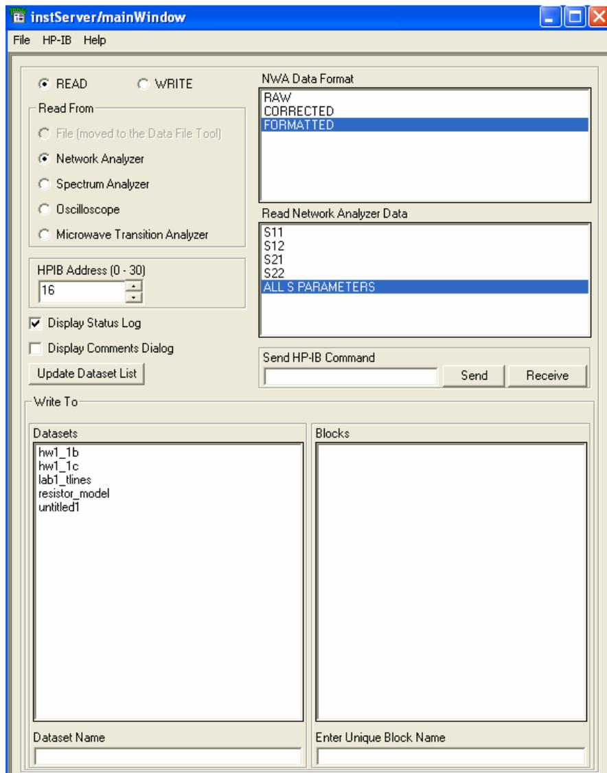
2. Initialize the GPIB card. Drag mouse over HP-IB on the tool bar and select Symbolic Name.
