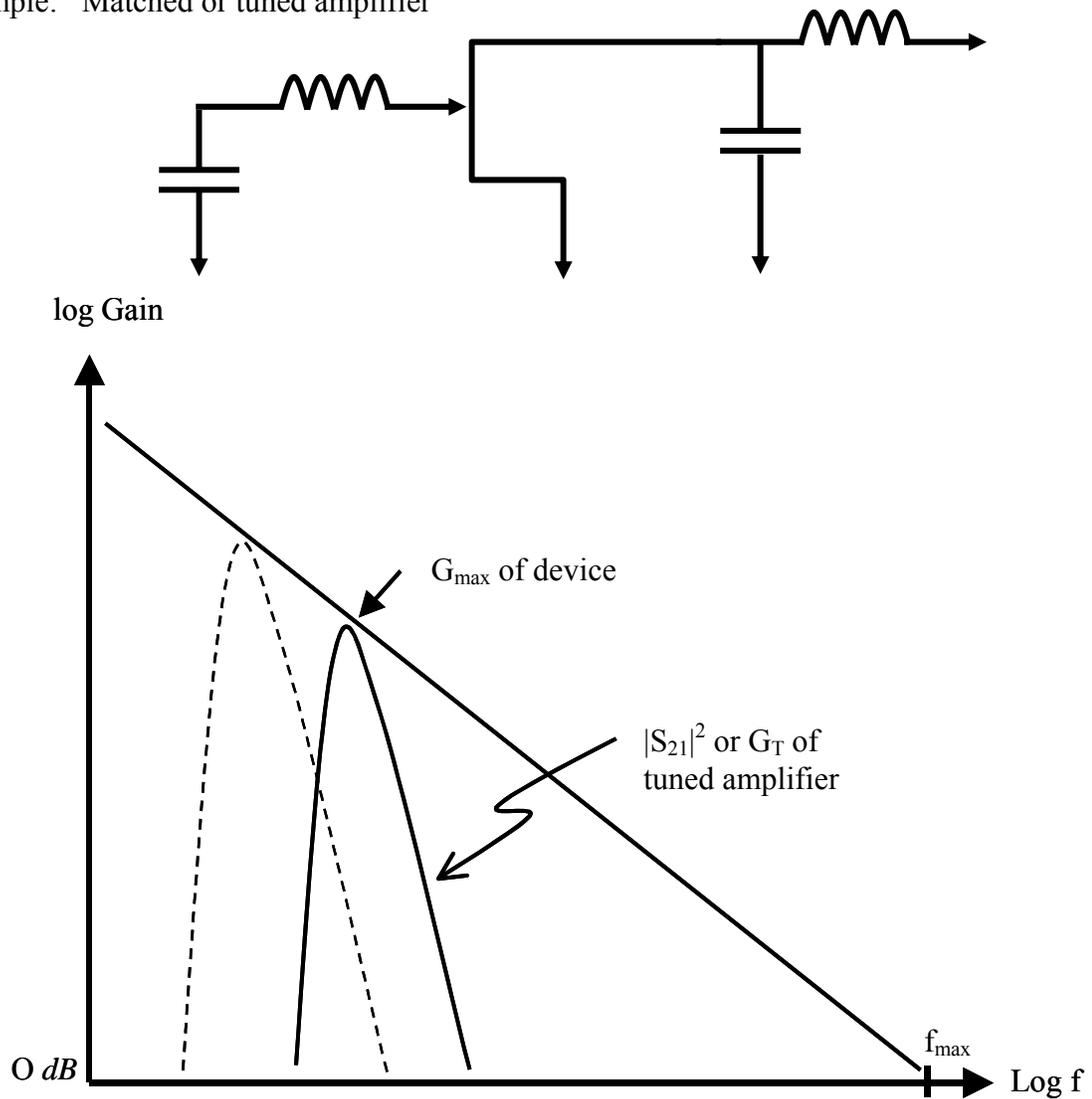
$G_{\max}$  is desirable for a tuned system (radio, receiver, etc.) Note that  $G_{\max}$  is a function of frequency.  $f_{\max}$  is the intersection with 0 dB gain – sometimes called the maximum frequency of oscillation. We see that a tuned amplifier (with frequency dependent matching networks) can achieve  $G_{\max}$  at only one frequency. A distributed amp, as discussed earlier, can achieve  $G_{\max}$  (at its highest frequency of operation) over a wide range of frequencies.
