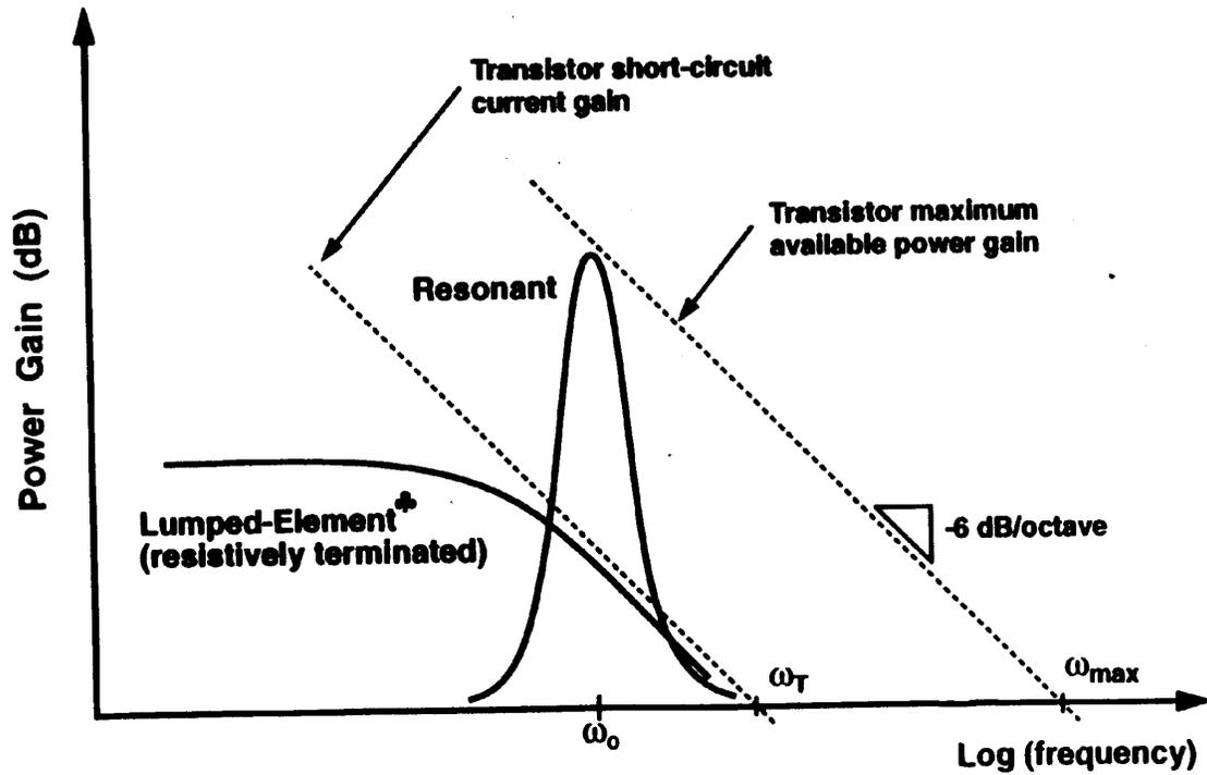
\* Bandwidth limited by device input capacitance.
