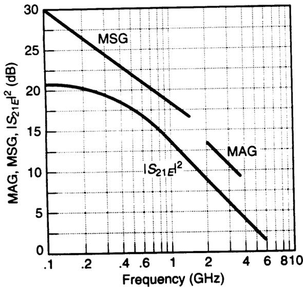
**Figure 3.6.2** Typical MAG (i.e.,  $G_{A,max}$ ), MSG (i.e.,  $G_{MSG}$ ), and  $|S_{21E}|^2$  versus frequency at  $V_{CE} = 18$  V and  $I_C = 30$  mA for the HXTR-5103. (From HP Microwave and RF Designer's Catalog 1990–1991; courtesy of Hewlett Packard.)
