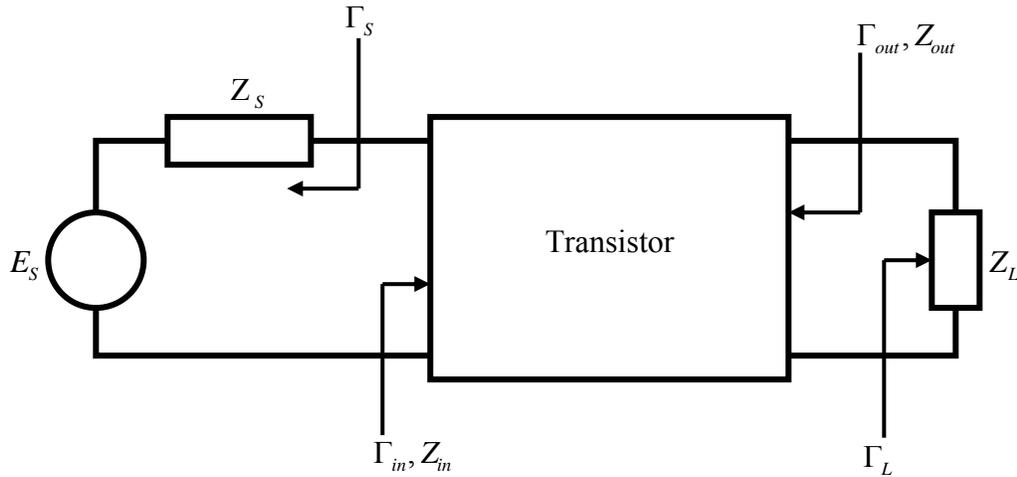
Oscillation is possible if either input or output port has a negative resistance. If a net negative real part exists, that is if  $\text{Re}\{Z_s + Z_{in}\}$  or  $\text{Re}\{Z_{out} + Z_L\} < 0$ , the transient response will grow and oscillation will occur.
