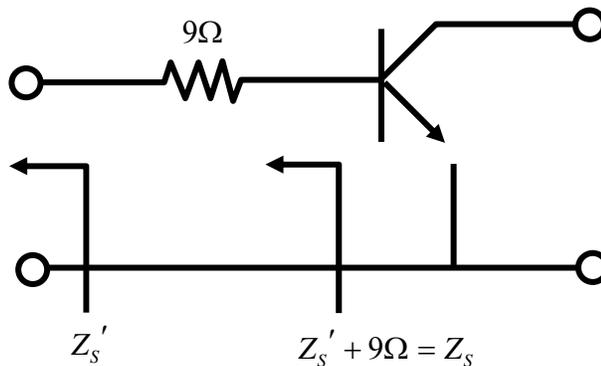
$\text{Re}(Z_s)$  is always  $> 9\Omega$ , so the unstable part of the  $\Gamma_s$  plane cannot be accessed for any  $\Gamma_s$ .
