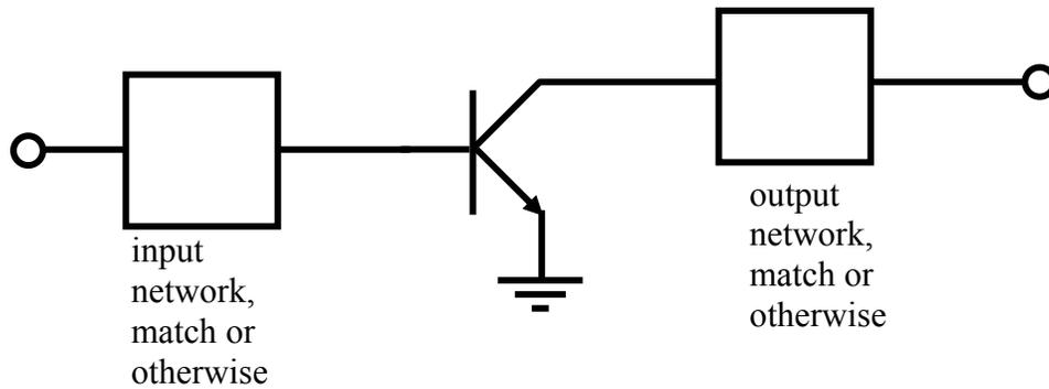
overall power gain must be  $\leq G_{\max}$ . This is called the *Maximum Available Gain*.
