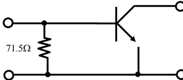
Output Stabilization: same procedure only on the  $\Gamma_L$  plane.
