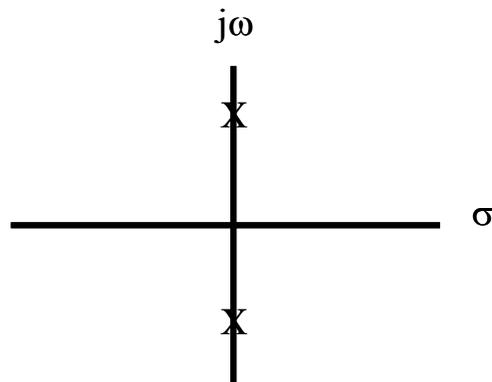
The transient response then has the form  $e^{j\omega t}$ , a sustained sinusoidal oscillation.
