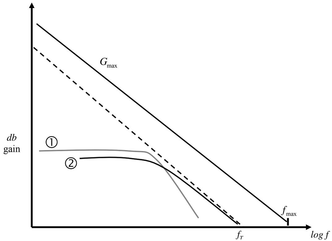
The gain-frequency curve clearly has to lie under the  $G_{\max}$  curve. In fact, the gain-frequency curve may be constrained well below this by the  $(f_T / f)^2$  line, or even lower.
