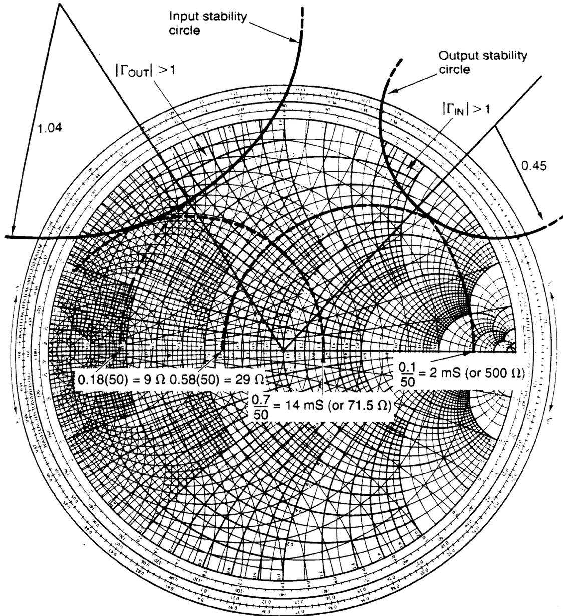
Figure 3.3.7 Input and output stability circles.
