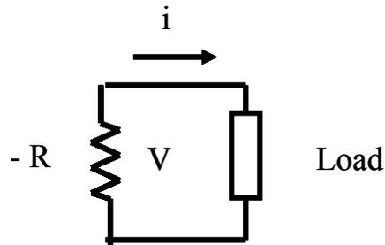
Note that the negative resistor has the opposite to the passive sign convention. Thus, it delivers power into the load rather than dissipating power as a positive resistor does.
