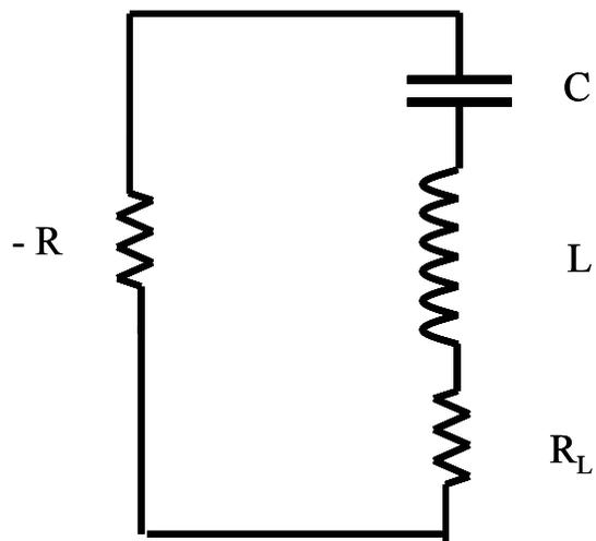
If  $|-R| = R_L$ , there is no net resistance in the loop. This locates the complex poles right on the  $j\omega$  axis.
