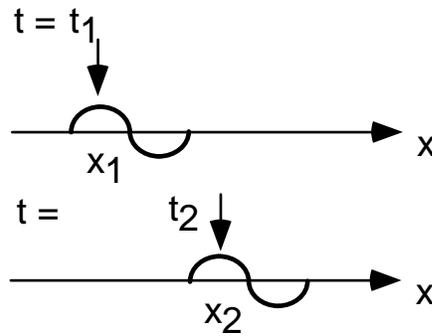
FIG. 3. Plot of wave propagation in the forward direction at times  $t_1$  and  $t_2$ .
