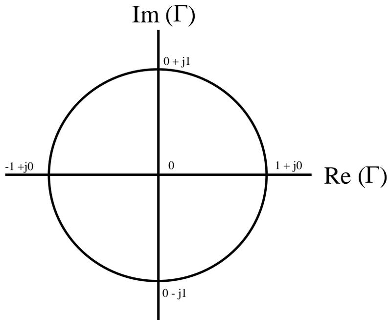
As we move away from the load by a distance  $\ell$  on the transmission line,  $\Gamma$  rotates by an angle  $\Delta\theta$  where:
