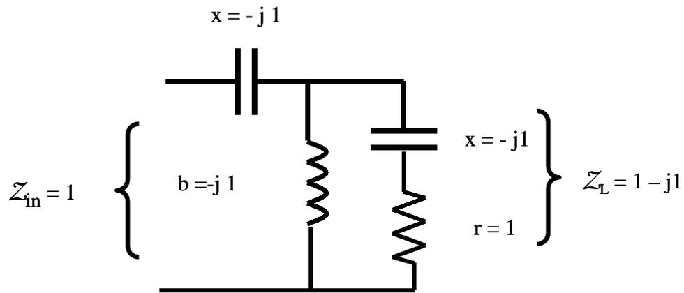
From our previous example, we proceeded from  $Z_L$  to  $Z_{in}$  by starting with  $Z_L = 1 - j1$ , taking into account the shunt admittance of the inductor by moving up on a constant conductance circle to the unit resistance circle, then down to the center through the series
