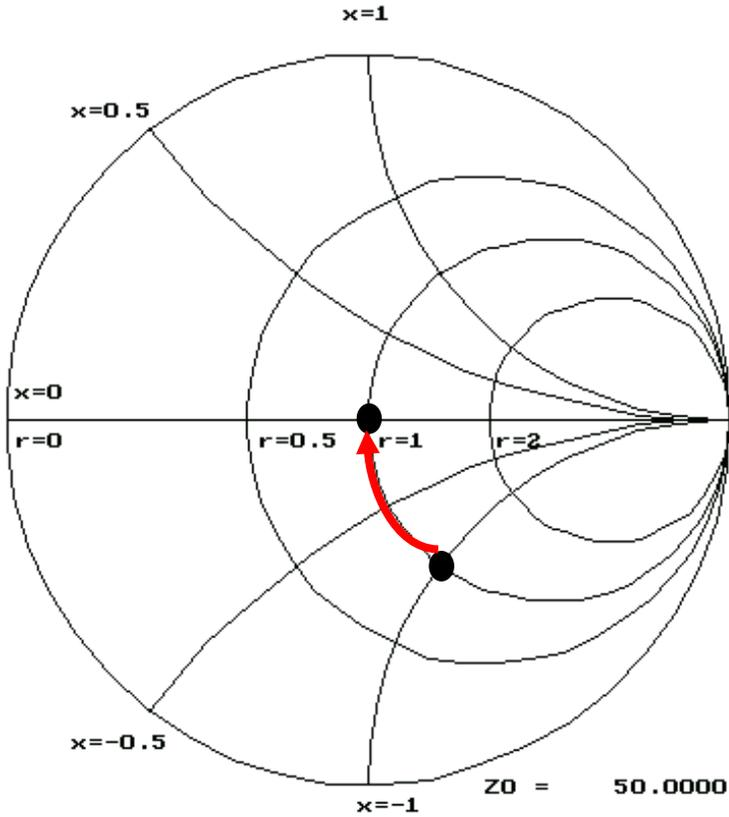
In this example, we have started with a series RC network,  $z = 1 - j1$ . By adding inductive reactance  $+ j1$  in series, we can again move along the  $r = 1$  circle up to the center of the chart.
