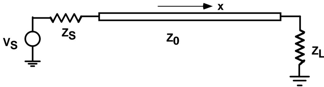
FIG. 1. Transmission line with impedance  $Z_0$  connects the source with Thevenin equivalent generator impedance  $Z_s$  to a load  $Z_L$ .
