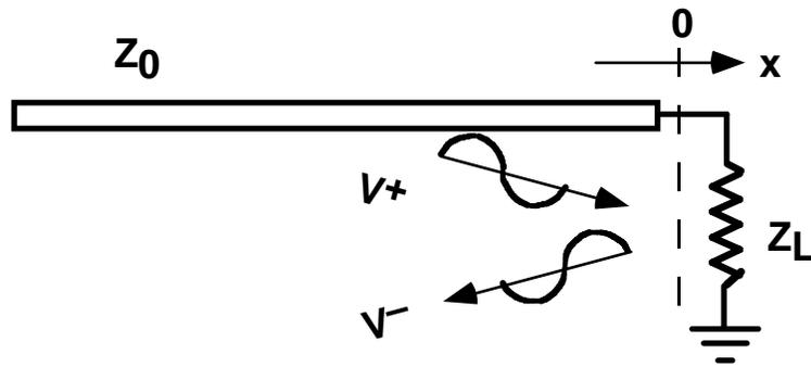
FIG 4. Reflection from a mismatched load impedance  $Z_L$ .
