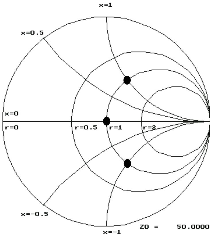
So, for example,  $z = 1 + j1$  represents a series RL network.  $z = 1 - j1$  is a series RC.  $z = 1$  is a point right in the center of the chart.
