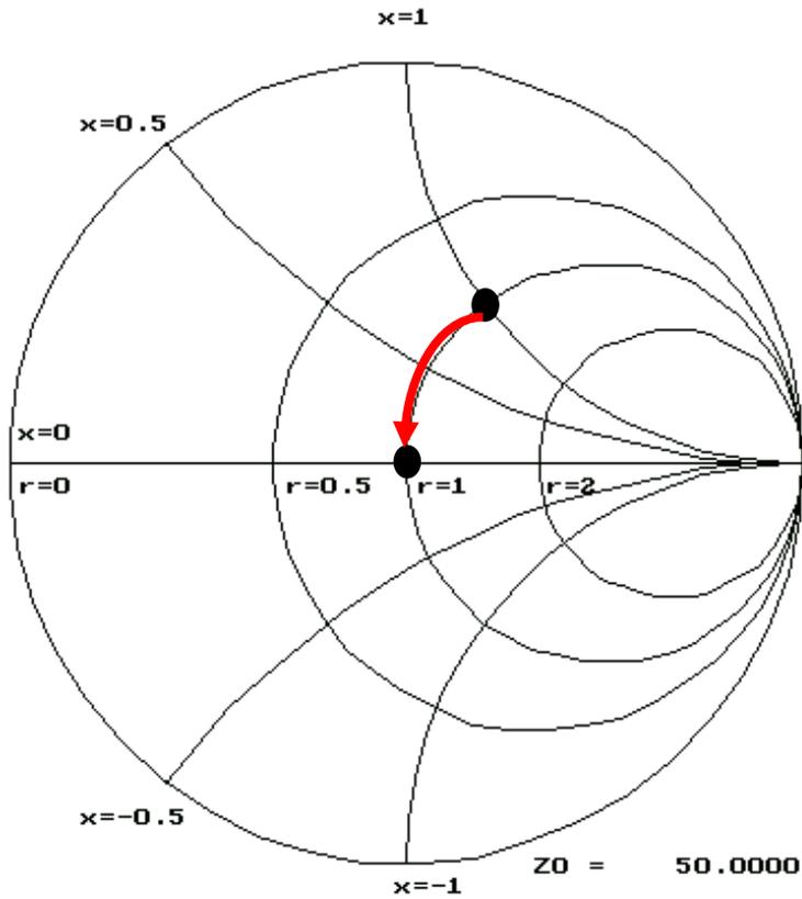
On this chart, we see an impedance  $1 + j1$  corresponding to the series RL network. If we add a capacitive reactance  $-j1$  in series with this, the point will move along the constant resistance line  $r = 1$  to the center. The reactance has been cancelled.
