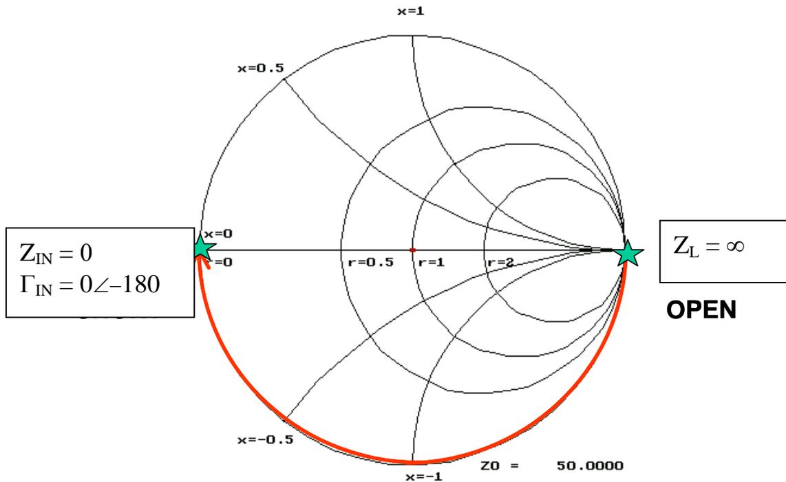
So, an open circuited quarter wave line produces a short circuit (when we ignore loss). Conversely, a shorted quarter wave line produces an open circuit.
