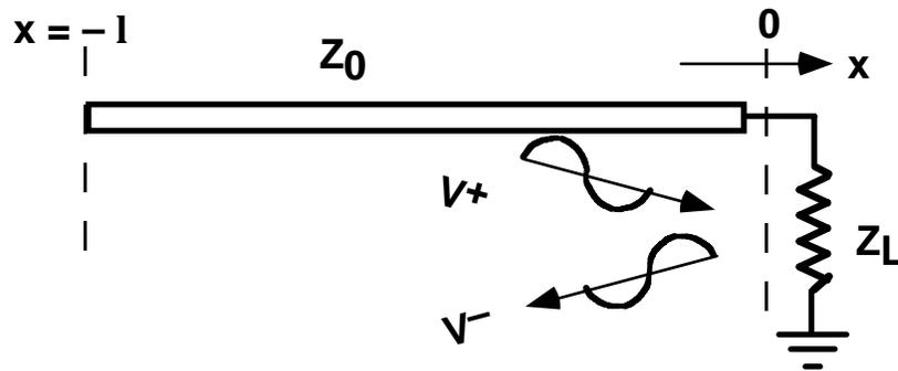
Now, we must determine voltage and current on the line as a function of position. This is often referred to as moving the reference plane. Here, we move from  $x = 0$  at the load to  $x = -l$  at the left end of the drawing.
