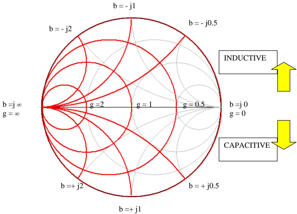
The impedance Smith chart is convenient for evaluating the effect of adding components in series. The admittance chart is useful for components in parallel.
