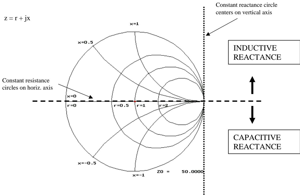
Note that the units of  $r$  are normalized to  $Z_0$ , in this case 50 ohms. So, the circle labeled  $r = 0.5$  corresponds to the 25 ohm resistance circle in this case. But,  $Z_0$  can be any convenient real value. If  $Z_0$  were 100 ohms,  $r=0.5$  would represent 50 ohms.
