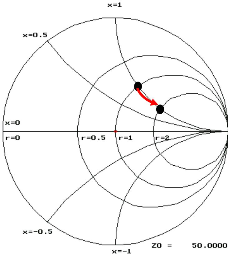
Series resistance. The chart can also represent the addition of resistance. This will correspond to movement along a circle of constant reactance. For example, if we begin with  $z = 1 + j1$  again and add a normalized  $r = 1$  to that, we arrive at  $z = 2 + j1$ .
