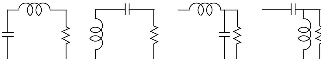
In addition to the problem of matching a purely resistive load that is not equal to  $Z_0$ , the typical practical problem includes substantial load reactance as well. As we shall see, this limits the bandwidth over which a good match can be achieved.
