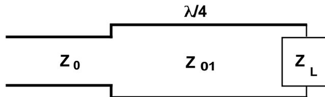
The bandwidth of such a matching transformer depends upon the ratio of  $Z_L/Z_0$ , which is the load impedance normalized to the desired input impedance. The reflection coefficient is approximately
