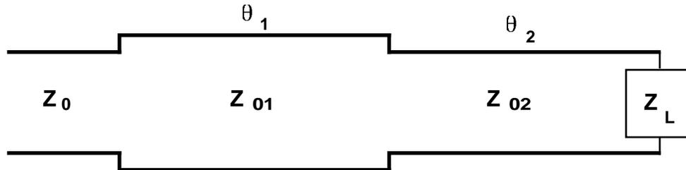
A more generally useful matching network can be realized by the use of two short sections of transmission line, of differing impedances. For the case of  $Z_02$  substantially higher than  $Z_L$  (say,  $Z_02 > 3|Z_L|$ ) and  $\theta_2$  small compared to a wavelength ( $\theta_2 < \pi/6$ ), the higher impedance section can be approximated to a series inductive reactance of
