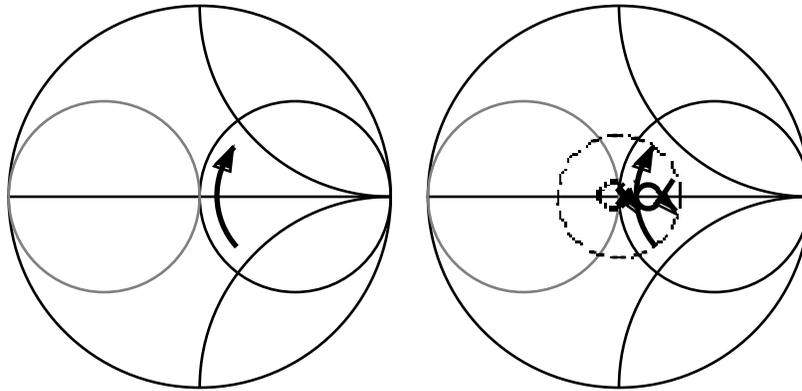
In order to reduce the SWR over the bandwidth shown, it is possible to place a resonant circuit across the terminals of the impedance, or to feed the impedance through a half-wave line of suitable  $Z_0$ . In either case, the operation of the matching network is to close up the arc of the impedance plot, resulting in a smaller range of SWR.
