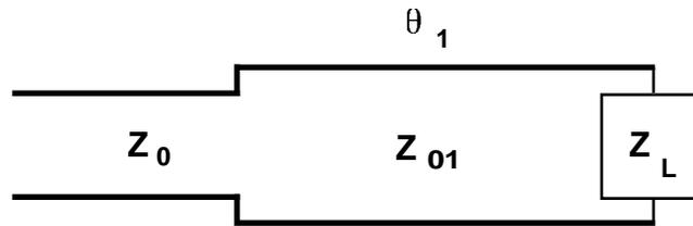
For  $Z_L = R + jX$ , we can obtain a match with the above circuit under the following conditions:
