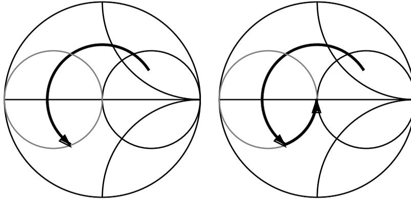
Although inconvenient to realize in transmission line format, there are two other solutions that are obtained by rotating the arbitrary impedance until it is on the 50Ω circle, then adding the proper series reactance to bring the resulting impedance to the 50Ω point.
