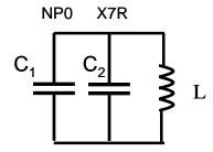
The equation below shows how the TCs of individual components combine<sup>1</sup>. Suppose that the inductor was resonated with a drift free capacitor (NP0). The frequency drift will be – 25 ppm/C. If the design frequency is 100 MHz, this corresponds to a drift of 2.5 kHz/C. But, the equation shows that you can set the total frequency TC (TCF) of a circuit to zero by combining capacitors with different TCs.
