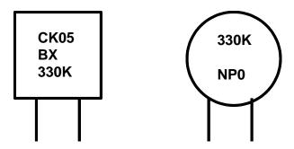
The two leaded capacitors above illustrate the labels found on typical capacitors of the X7R and NP0 types. The value is given by the numerals: 330. In this example, this is 33 pF. It goes  $1^{st}$  significant digit (3),  $2^{nd}$  significant digit (3), and multiplier ( $10^{0}$ ). The letter K is the tolerance, which is  $\pm 10\%$ .
