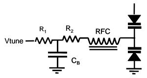
The varactor diode TC is shown on the data sheet – roughly +250 ppm/°C. This is an unacceptably high TC for the entire resonator, however, the varactor provides only a small part of the total capacitance. You should implement the fixed capacitors in the resonator with zero TC (NP0) capacitors. The inductor core material has a TC of 0 ppm/°C.
